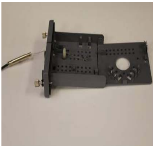
Figure 25. Putting the Thermocouple into the column cartridge
