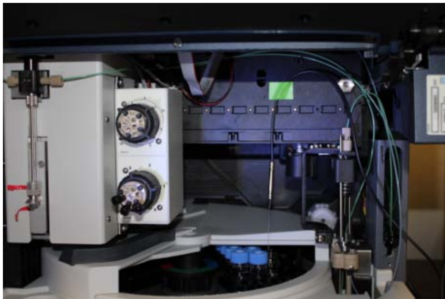
Figure 27. Temperature sensor inserted into the vial
