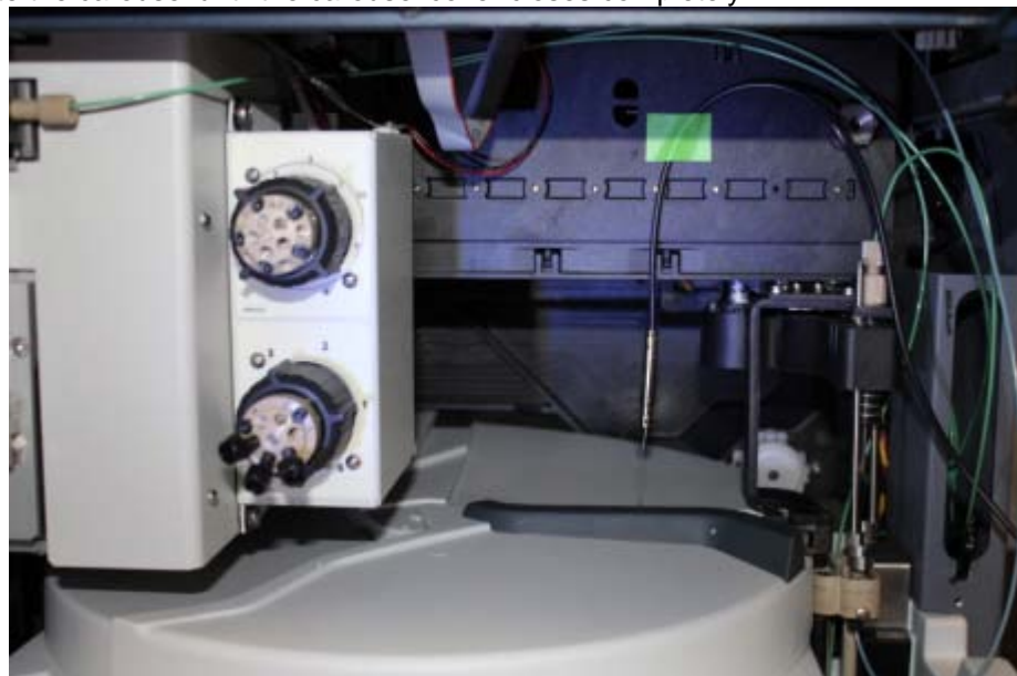
Figure 28. Temperature sensor inserted into the vial
