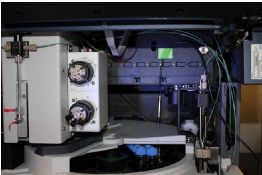
Figure 31. Temperature sensor inserted into the vial
