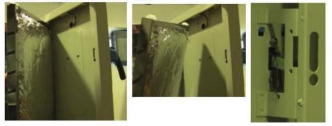
Unscrew the front door handle with a box spanner / socket wrench, size XX, to loose the door handle.
