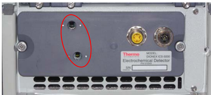
Figure 61. ED cell mounting location
