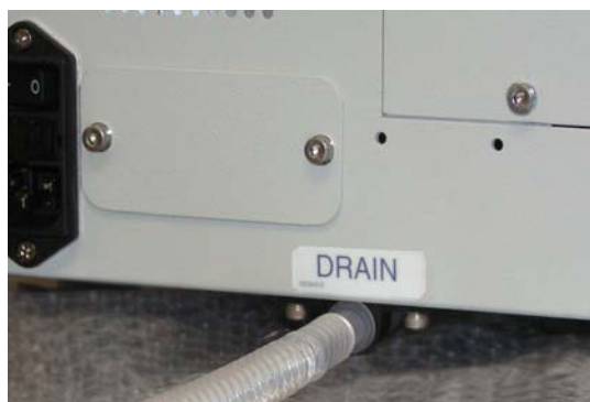
Figure 22. Drain port with drain line attached
