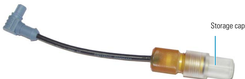
Figure 60. pH-Ag/AgCl reference electrode in storage cap
