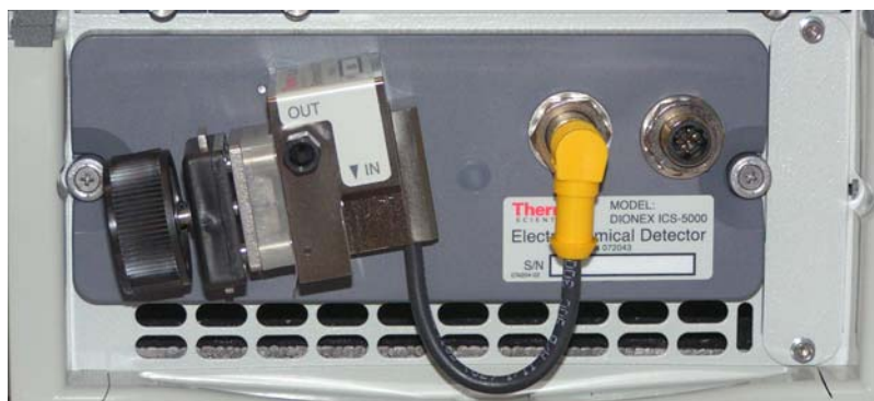
Figure 62. ED cell installed on the detector
