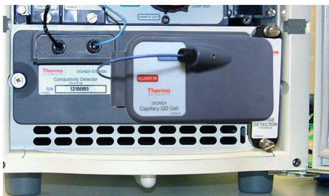
Figure 48. QDC mounted on the CD and QD
