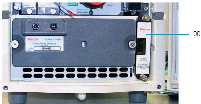
Figure 16. CD and QD installed in compartment
