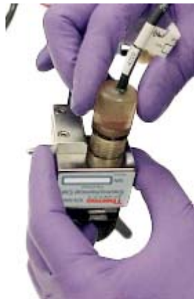
Figure 66. pH-Ag/AgCl reference electrode O-ring in the reference electrode well
