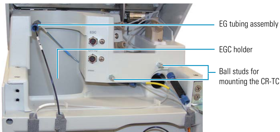
Figure 9. Front tray before installing EGC and CR-TC
