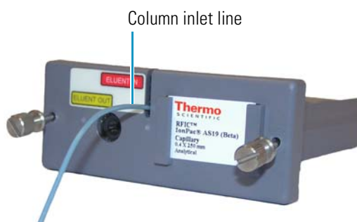
Figure 40. Column cartridge closed; with column inlet line routed through slot
