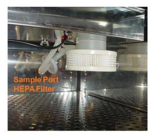
Access port should be fitted with an **Access Port Filter Assembly** and not a solid stopper. Part number **(190985).**
