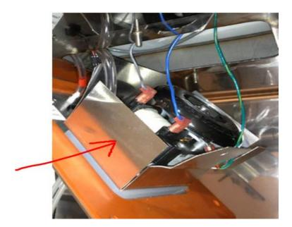
A unit without a metal shield will result in condensation forming on the chamber ceiling. This is due to the blower wheel forcing cooler air down onto the chamber ceiling. This will create a "cool" spot and condensation will develop in a high RH environment.
