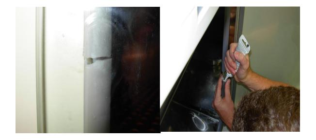
Inoperative inner door heater. This can be caused by a poor or broken connection at door heater harness connection or blown door heater fuse on main pcb. Fuse (F1) 3.5A
