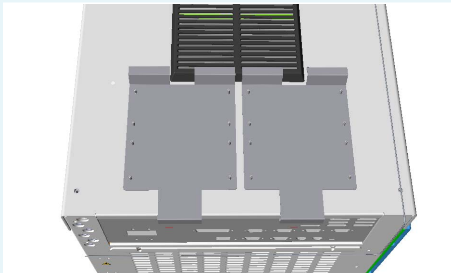
Figure 484. Installation of Four PDD Detectors
