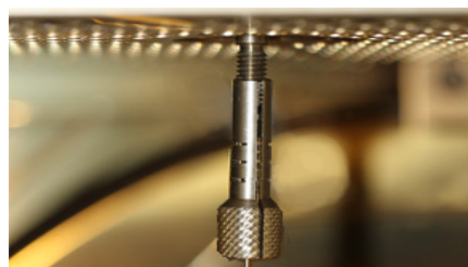
Figure 380. Securing the 30 cm Fused Silica Restrictor to the No-Vent Microfluidics Module
