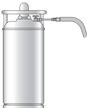
Figure 16. Liquid Nitrogen Tank Configuration
