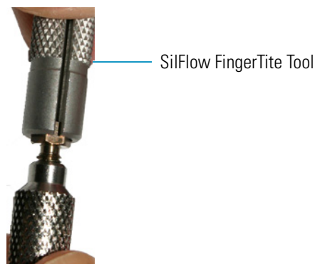
Figure 388. Swaging the Ferrule Using the SilFlow FingerTite Tool
