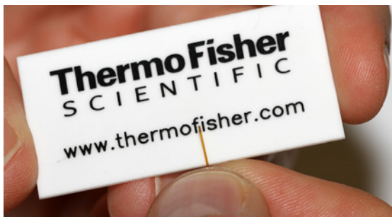
Figure 386. Cutting the Column with the Scoring Wafer
