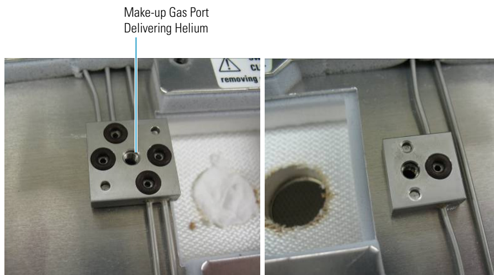
Figure 468. Confirming Presence of O-rings
