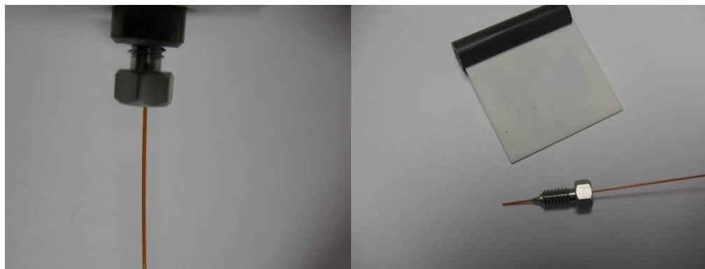
Figure 474. Installing the Column in the Injector
