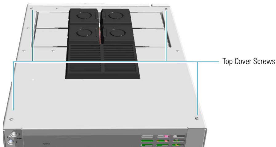
Figure 182. Top Cover Removal (1)
