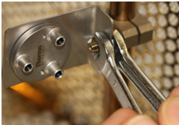
Figure 378. Securing the Holder for the Microfluidics Splitter
