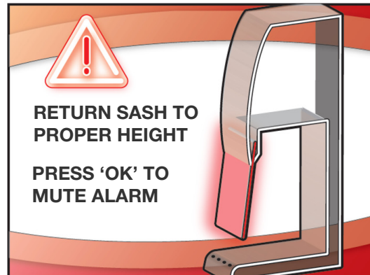
Figure 17. Sash height alarm
