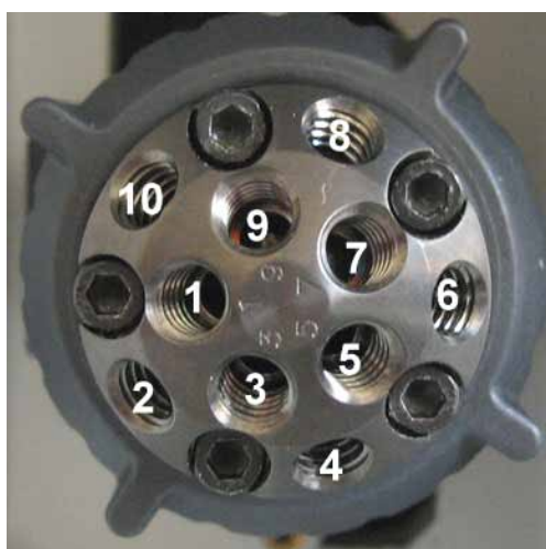
Fig. 27: Example for the connections on a 2-position, 10-port column switching valve
