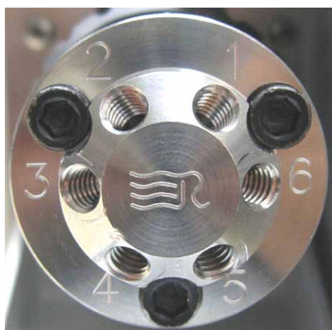
Fig. 26: Example for the connections on a 2-position, 6-port column switching valve
