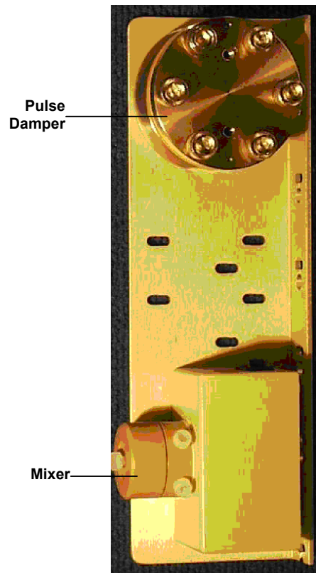
Figure 3-5: The Mixer and Pulse Damper Mounted on Support Bracket
