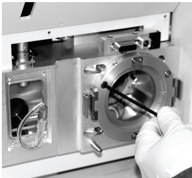
Figure 50. Removing the ion optics cage assembly retaining screws
