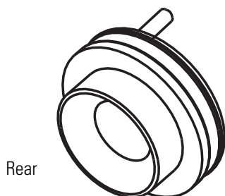
Figure 16. Tube lens of the TSQ Quantum Access, TSQ Quantum Access MAX, or TSQ Quantum Ultra
