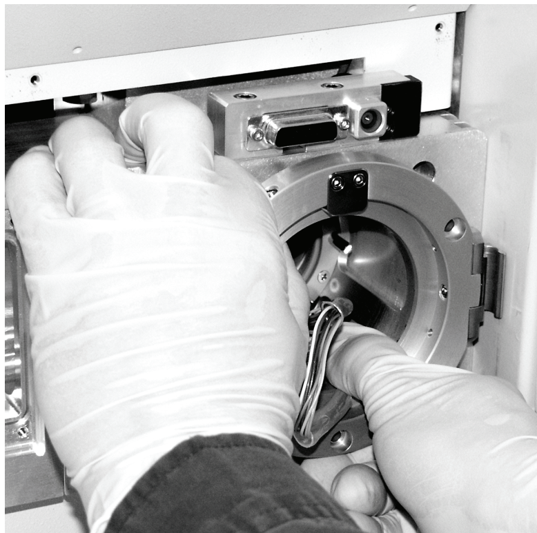
Figure 52. Removing the ion optics cage assembly
