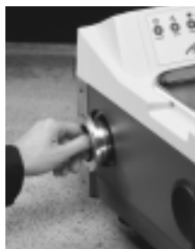
Figure 1. Changing the source assembly on an Antaris FT-NIR analyzer
