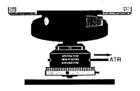
9. Put the slide selector into the *ATR* mode and raise the Sample Stage using the Z-focus adjustment knob.
