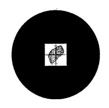
8. Still in *Survey* mode, focus and center the sample area of interest in the field of view using the x and y adjustment knobs for the Sample Stage.
