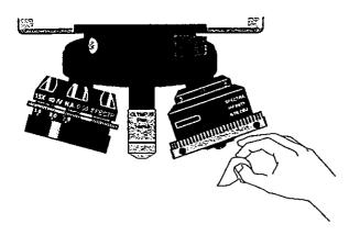
Rotate the nosepiece so that the ATR crystal is accessible. Wipe the crystal with lens tissue. Water or isopropanol may be used to clean the crystal.
