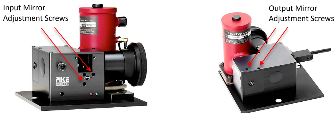
Figure 3: Locations of mirror alignment ports
