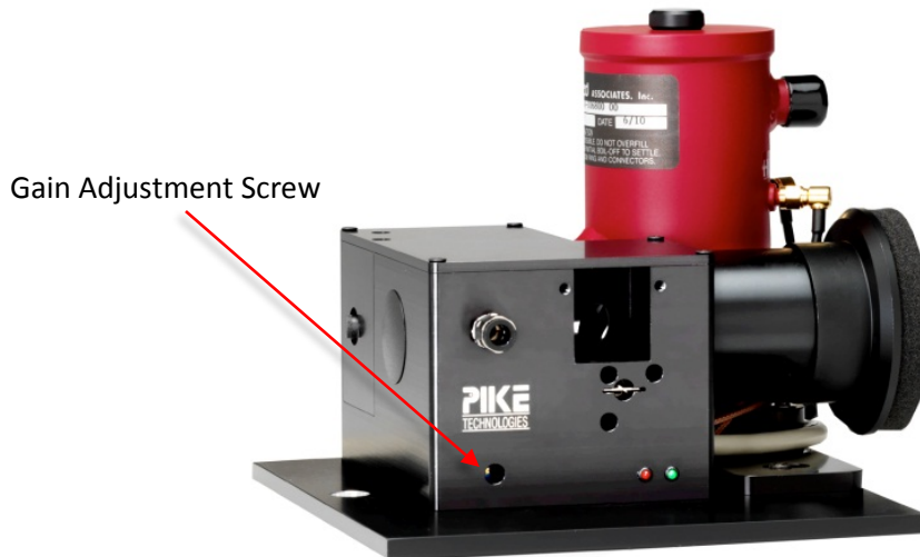
Figure 5: Illustration of MCT detector alignment point
