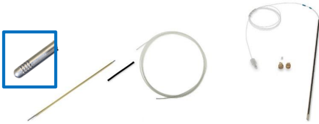
FIGURE 10 Stainless Steel Probe for Oils Applications (Left) and Carbon Fiber Probe for Aqueous Applications (Right)
