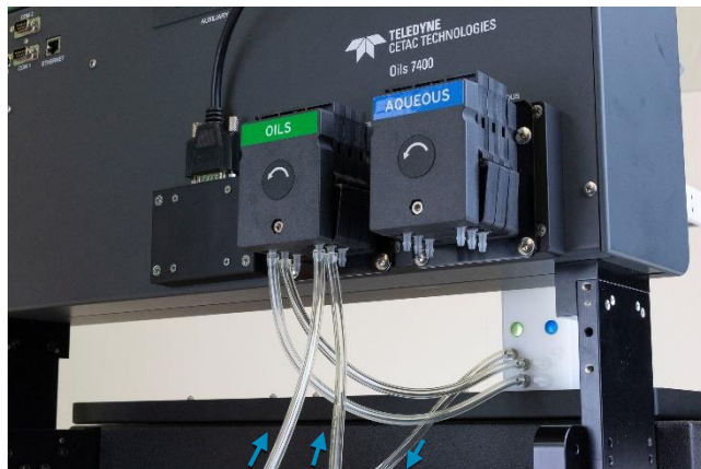
From Rinse Solution Source To Waste Container
