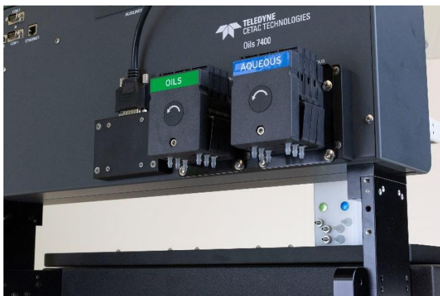
FIGURE 15 Autosampler Before Rinse Tubing Connections
