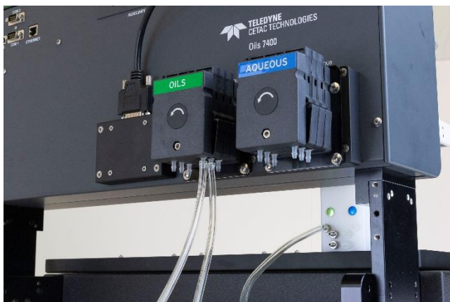
FIGURE 17 Connecting the Rinse Supply to the Pump
