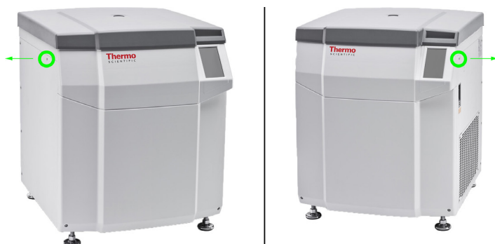
Figure V-2: Position of the mechanical emergency door release
