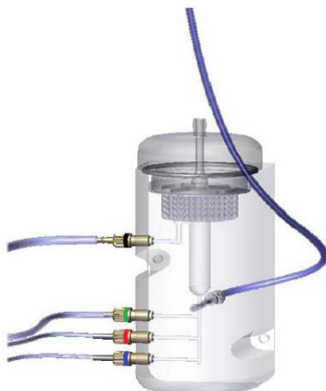
Figure A-3. Integrated hydride generation accessory
