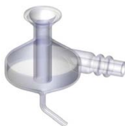
Figure 3-8. Baffled cyclonic spray chamber
