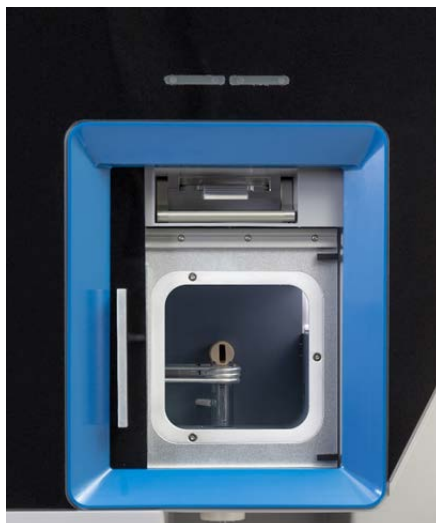
Figure 8-3. Access to torch box
