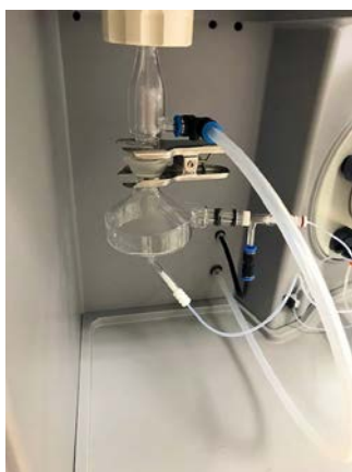
Figure A-8. Spray chamber and sheath gas adaptor
