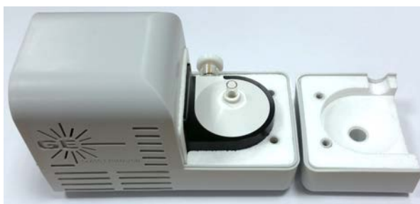
Figure 3-10. IsoMist™ XR - temperature controlled spray chamber
