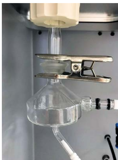
Figure A-5. Spray chamber and the spray chamber adaptor
