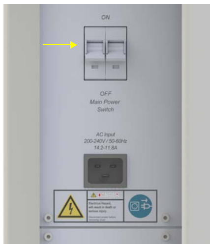
Figure 6-1. Main power switch of iCAP PRO Series ICP-OES
