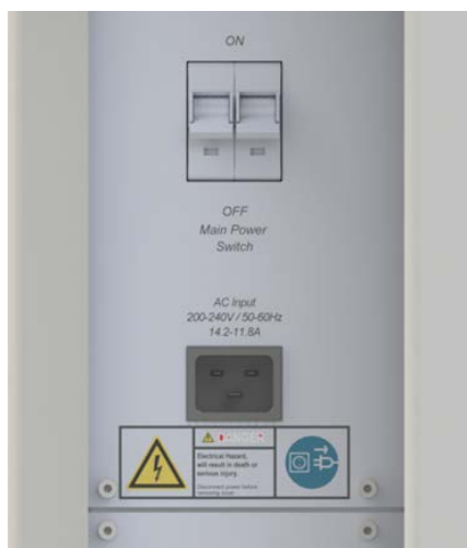
Figure 5-13. Power connection at rear panel of iCAP PRO Series instrument
