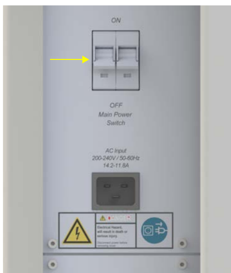
Figure 4-3. Power switch of iCAP PRO Series ICP-OES
