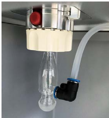
Figure A-6. Sheath gas adaptor inserted and connected
