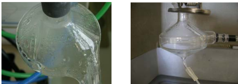
Figure 8-2. Spray chamber: dirty (left) - clean (right)
