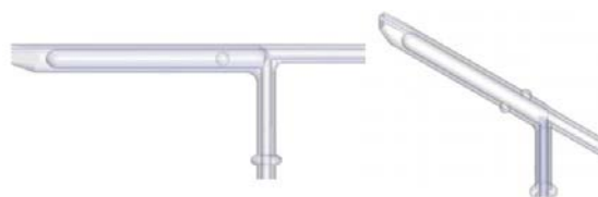
Figure 3-9. V-groove nebulizer for heavy organic sample analysis
