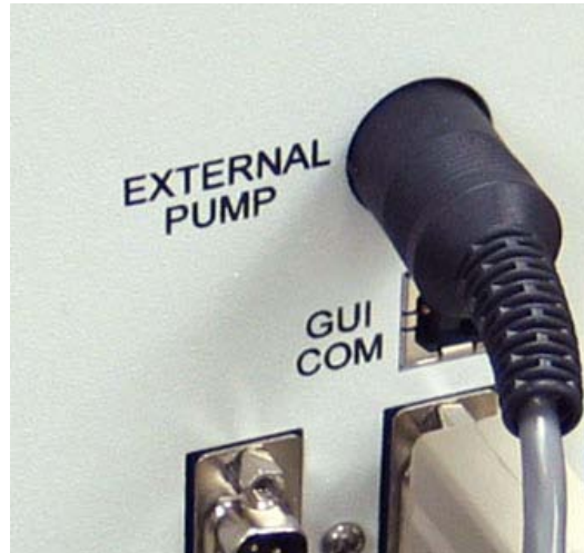
Figure 7-3 Connecting the External Pump to the Electronics Module
