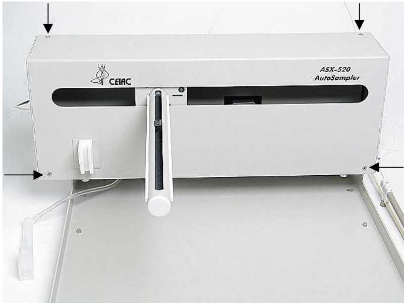
Figure 4-16 Front View of ASX-520 Autosampler Showing Front Cover Screws
