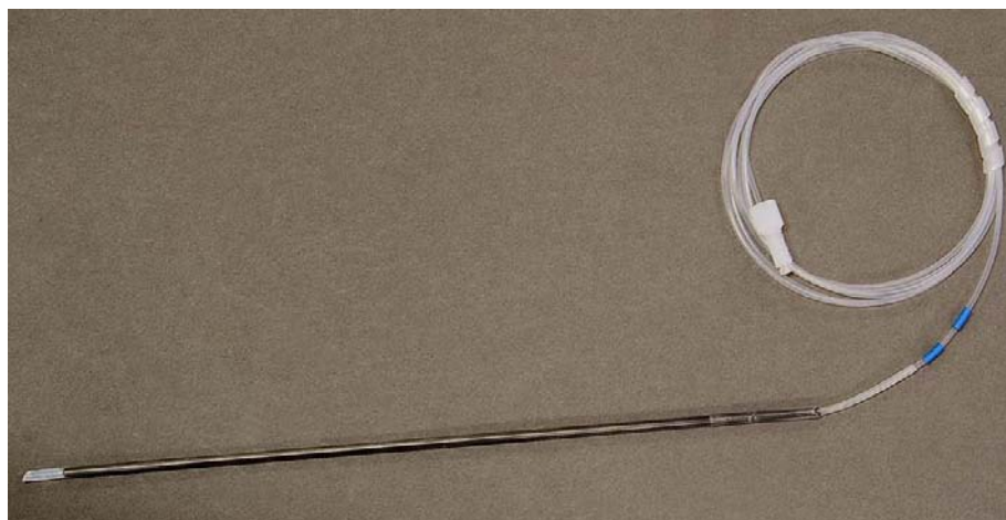
Figure 4-10 Double Blue Bands Identify the 1.0mm I.D. Sample Probe ( carbon fiber probe shown is standard equipment )
