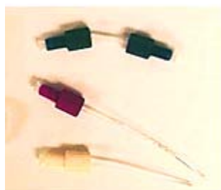
Figure 6-7 Tubing for the Standard Addition Mixing Tee
