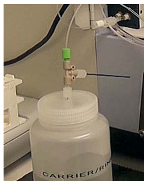
Figure 6-12 Passive Bubbling Tee in Rinse Solution Bottle
