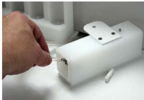
Figure 5-4 Removing the Rinse Tubing
