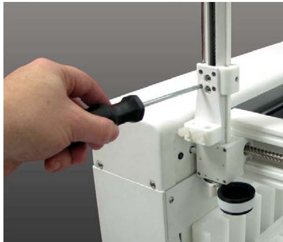
Figure 5-16 Removing the Plate
