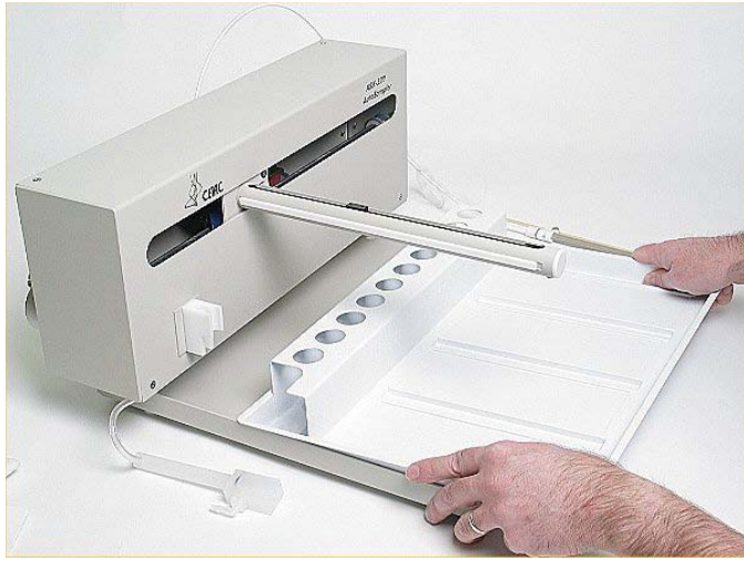
Figure 4-15 Removing the Tray (ASX-520)
