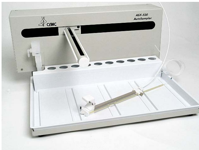
Figure 4-12 Z-Drive Removed from Arm Assembly. (Photo shows standard ASX-520 tray with integral standards rack.)
