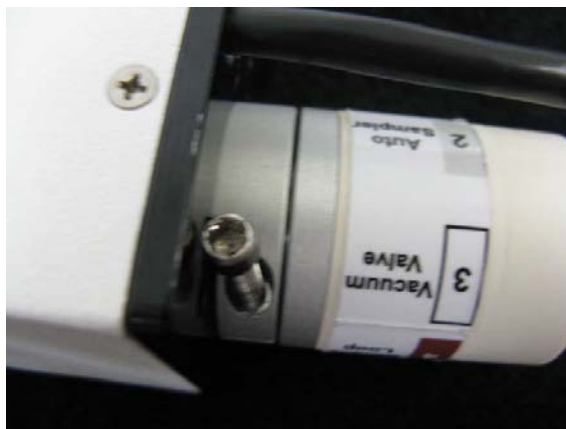
Figure 11-5 Locking collar with hex screw loosened
