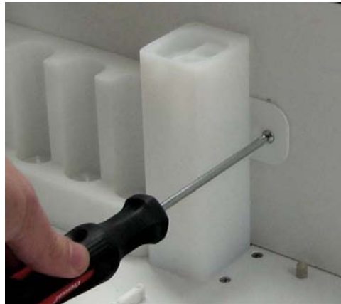
Figure 5-2 Removing the Rinse Station Screw
