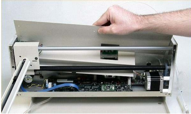
Figure 4-19 Removal of Inner Shield (ASX-520)
