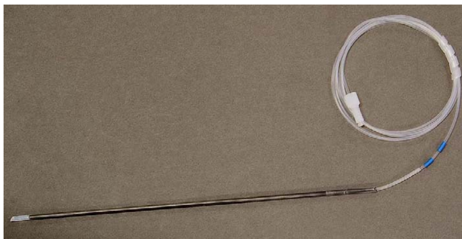
Figure 3-5 Double Blue Bands Identify the 1.0mm I.D. Sample Probe (carbon fiber probe is shown)
