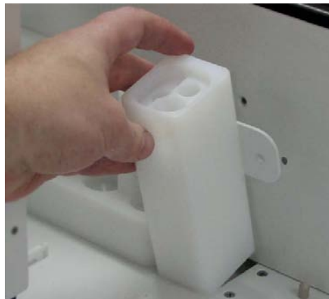
Figure 5-3 Removing the Rinse Station
