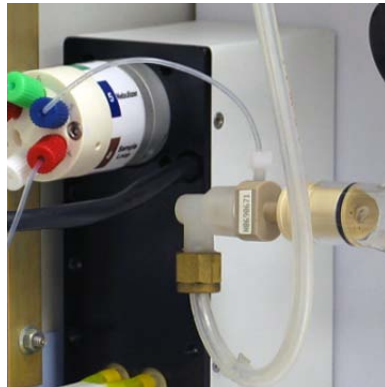
Figure 6-5 Nebulizer Connected to Port #5
