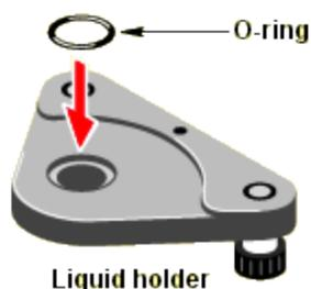
2. Align the pin on the bottom of the liquid holder with the alignment hold on the sampling plate.
