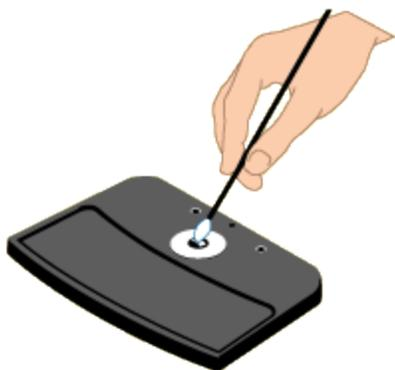
Dry them with unscented tissues or cotton. If you clean the crystal with a solvent, allow enough time for the solvent to evaporate completely. To ensure complete evaporation, dry the crystal with clean, dry air or nitrogen.
