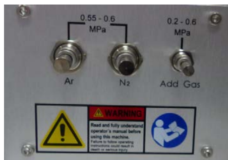
Figure 3-12. Connections on the instrument for gas supply
