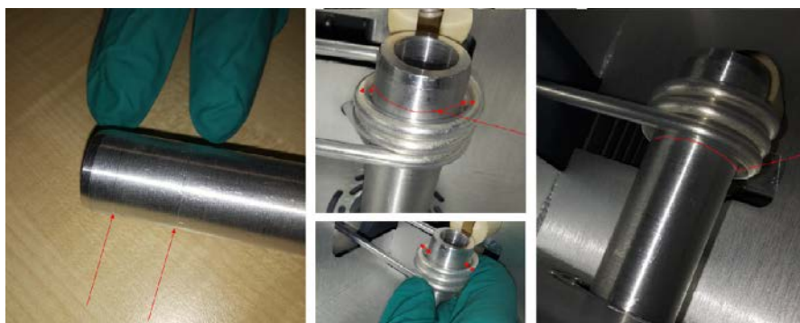
Figure 10-1. Metal torch dummy with alignment marks (left) and relative coil positioning (right)
