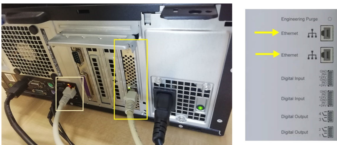
Figure 4-1. Network connections to local network onboard (left) and instrument to network card (right)
