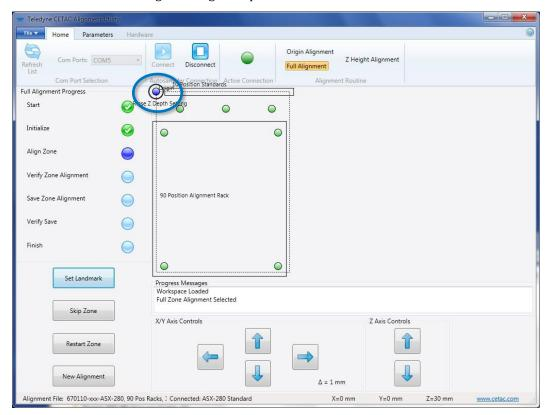
21 The tip of the probe will move into the rinse station. No additional action is required except to click **Set Landmark**, then click through the prompts (**Yes**, **Write Zone**, and **Yes**) to save the alignment.
