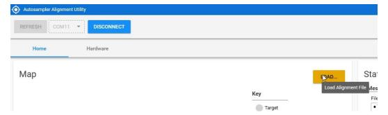
Choose the alignment file that matches the number of rack positions and tray standards positions for your autosampler. You will need to browse for the alignment files which are located on the CD in the Alignment Documents folder, then in the Alignment Files folder, or they can also be requested through the Teledyne CETAC website at <a href="https://www.teledynecetac.com">https://www.teledynecetac.com</a>.
