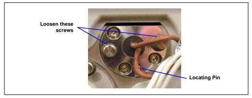
Figure 5-6. Tungsten Lamp Screws and Locating Pin
