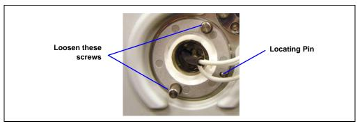
Figure 5-3. Deuterium Lamp Screws and Locating Pin
