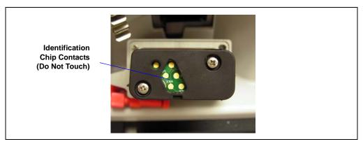
Figure B-3. Rear of Flow Cell with Identification Chip Contacts
