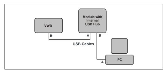
Figure B-12. Example USB Connection: Dionex VWD Connected to Another Module in the System
