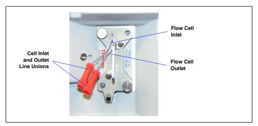
Figure B-4 shows the flow cell after installation is complete.
