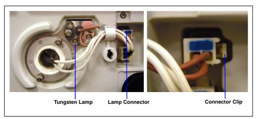
Figure 5-5. Tungsten Lamp, Connector, and Clip
