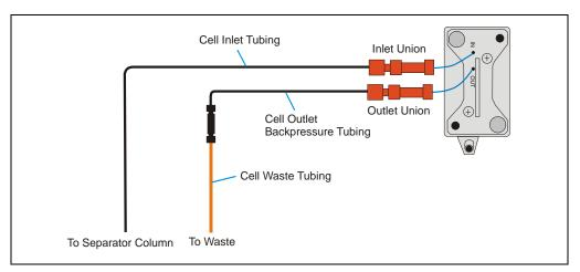
Figure B-5 is a schematic of the flow cell tubing connections.
