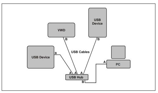
Figure B-13. Example Connections: Multiple Modules Connected via an External USB Hub
