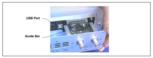
Figure B-10. Installing the DAC Plug-In Module
