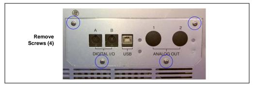
Figure B-9. Removing the DAC Access Panel
