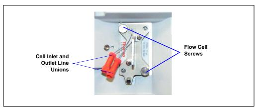
Figure 5-7. Removing the Flow Cell
