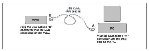
Figure B-11. Dionex VWD Connected Directly to the Chromeleon PC
