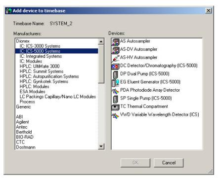
Figure B-15. Adding the Dionex VWD to a Timebase
