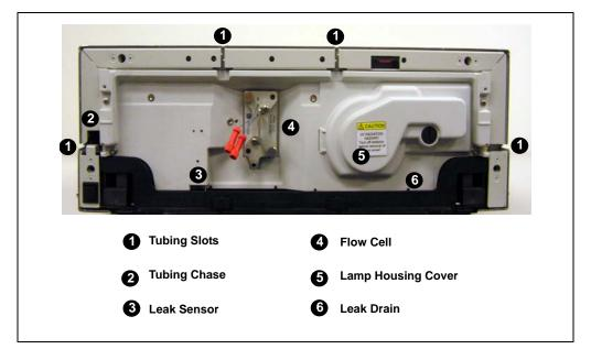
Figure 2-3. Dionex VWD Interior View (Front Cover Removed)
