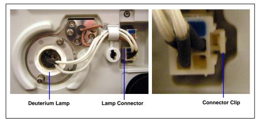
Figure 5-2. Deuterium Lamp, Connector, and Clip
