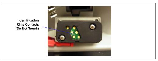
Figure 5-8. Rear of Flow Cell with Identification Chip Contacts
