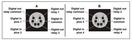
Figure B-7. 6-Pin Mini-DIN Digital I/O Ports
