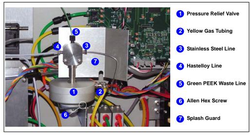
Figure 5-18. Connections to the Pressure Relief Valve
