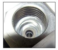
2. Place the new filter (P/N 067327) on top of the backup ring. Check that the filter is seated, lies flat, and is centered in the inlet gland.
