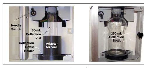
Figure B-12. Installing the Collection Vessel
