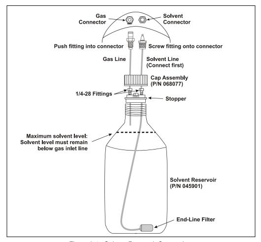
Figure 3-1. Solvent Reservoir Connections
