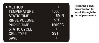
Figure 3-18. Method Editor Screen (All Parameters Shown)
