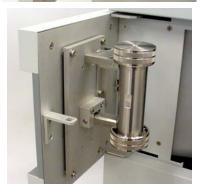
Figure B-11. Installing a Sample Cell
