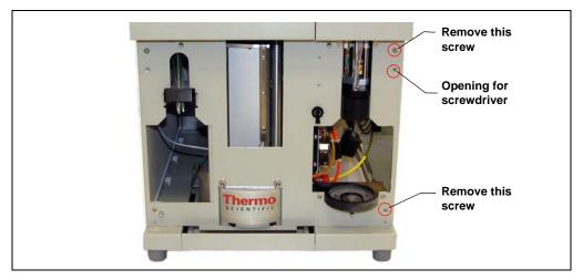
Figure 5-6. Inner Front Panel
