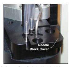
Figure 5-23. Removing the Needle Block Cover
