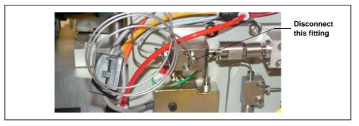
Figure 5-25. Disconnecting the Source Needle Fitting from the Static Valve
