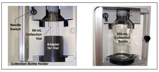
Figure 3-10. Installing the Collection Vessel
