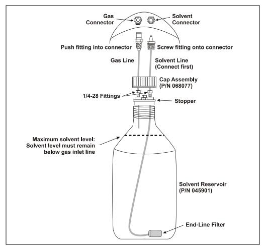
Figure B-4. Solvent Reservoir Connections (Top View)
