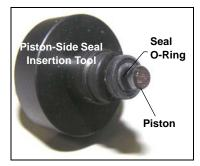
5. Rest your thumbs on the back of the tool and press down firmly (with equal pressure) on the left and right sides of the tool. When you hear a snap (indicating that the new seal is seated in the valve body), remove the piston and the tool from the valve body.
