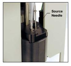
Figure 5-24. Removing the Source Needle from the Needle Block
