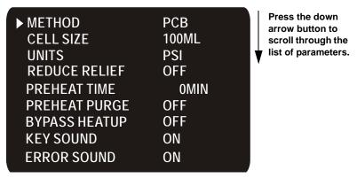
Figure C-4. Setup Screen (All Parameters Shown)
