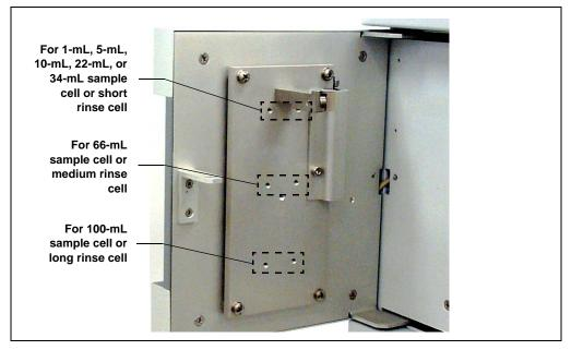
Figure B-7. Mounting Sites for the Cell Holder Lower Latch
