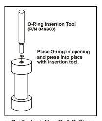
Figure B-10. Installing Cell O-Rings
