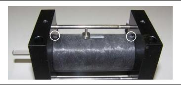
Figure 5-17. Alignment Marks on Pump Cylinder and End Plates
