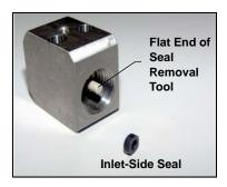
4. Insert the flat end of the seal removal tool into the inlet side of the valve body and push the seal out of the piston side of the valve body.
