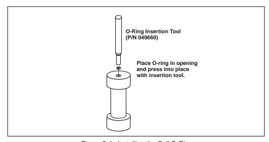
Figure 5-4. Installing the Cell O-Ring
