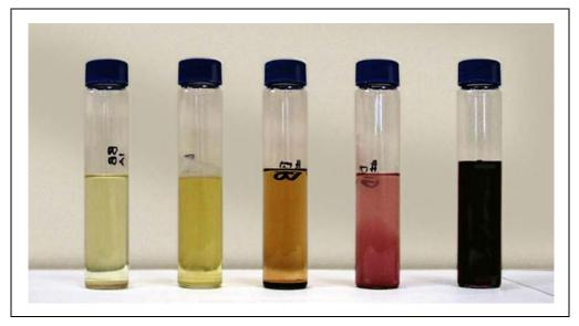
Figure E-3. Selectivity in ASE. The same sample of blueberries was extracted with hexane (most left), DCM, ethyl acetate, acetonitrile, and ethanol
