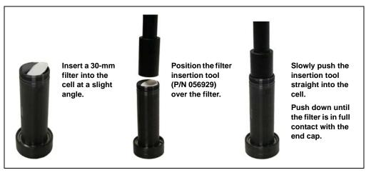
Figure 3-5. Installing a 30-mm Cell Filter in a 34-mL, 66-mL, or 100-mL Cell (Zirconium Cell Shown)
