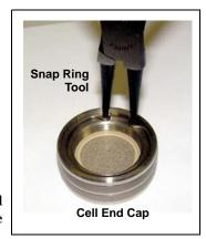
Figure 5-1. Removing the Snap Ring
