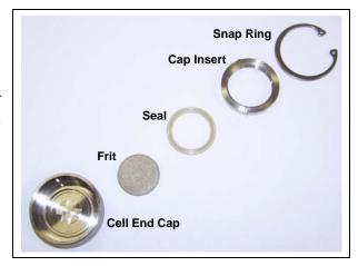
Figure 5-2. Cell End Cap Disassembled
