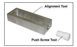
11. Place the alignment tool (P/N 068117) on top of the static valve.
