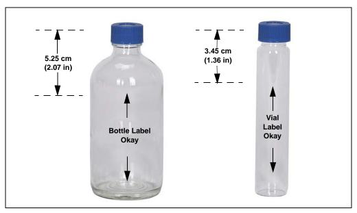
Figure 3-9. Placement of Collection Vessel Labels
