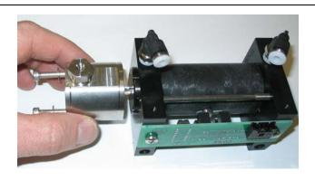
Figure 5-11. Removing the Pump Head
