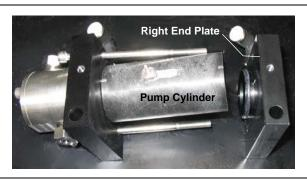
Figure 5-14. Removing the Pump Right End Plate
