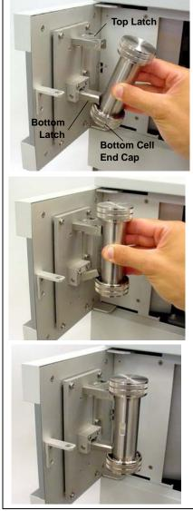
Figure 3-15. Installing a Sample Cell
