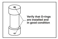
Figure B-9. Inspecting Cell O-Rings
