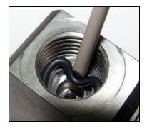
6. Using a cotton-tipped swab (or other tool with a soft tip), thoroughly clean the inside of the valve body. If necessary, moisten the area with IPA (isopropyl alcohol) or acetone to remove all debris, sediment, and precipitates.
