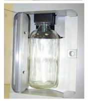
Figure 3-11. Installing the Waste Bottle
