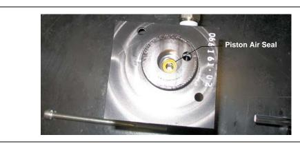
Figure 5-16. Removing the Piston Air Seal
