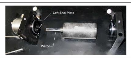
Figure 5-15. Removing the Pump Left End Plate
