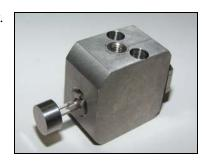
7. Slide the piston ferrule onto the piston holder at the end of the cylinder.
