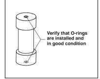
Figure 3-7. Inspecting Cell O-Rings
