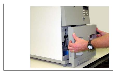
Figure 5-5. Removing the Lower Front Trim Panel
