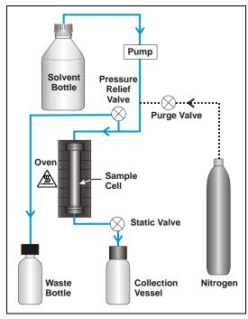
Figure 2-4. Extraction Process Schematic
