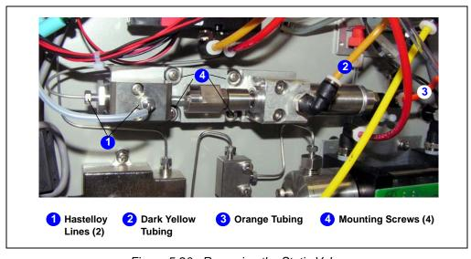
Figure 5-20. Removing the Static Valve
