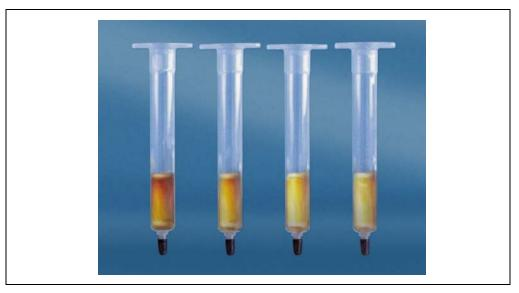
Figure E-4. Residual co-extractives after the ASE extraction of a coffee sample trapped on an SPE cartridge, the ASE cells containing from 0 to 6 g Florisil. From left to right: 1) No Florisil in the ASE cell, 2) 2 g Florisil in the ASE cell, 3) 4 g Florisil in the ASE cell, and 4) 6 g Florisil in the ASE cell.
