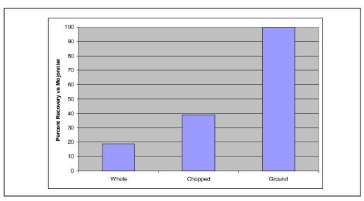
Figure E-2. Effect of Sample Particle Size for ASE vs. Mojonnier Extraction. Whole cheese (0.5 to 1.5 cm size); chopped (2-5 mm); ground (mixed thoroughly with diatomaceous earth)
