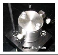
Figure 5-13. Removing the Pump PC Board and End Plate Bolts
