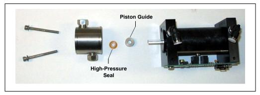
Figure 5-12. Replacing the Dionex ASE 150 Piston High-Pressure Seal
