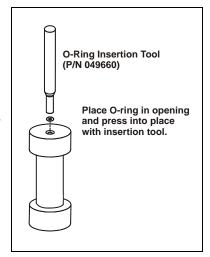
Figure 3-8. Installing a Cell End Cap O-Ring
