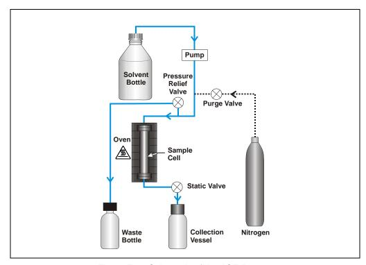
Figure E-1. Schematic of the ASE Process
