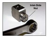
b. Remove the seal backup ring and the filter from the inlet side (they may fall out on their own). Save the seal backup ring. You can discard the filter.
