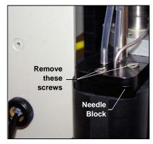
Figure 5-22. Removing the Needle Block Screws
