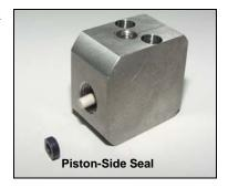
Insert the pointed end of the seal removal tool into the valve body.
