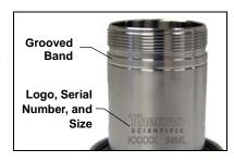
Figure 3-5. Sample Cell Top (Larger Cells)
