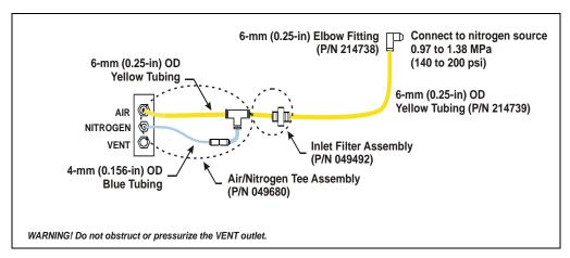
Figure B-2. Connections for Substituting Nitrogen for Air
