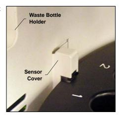
Figure 3-13. Cutout-Sensor Cover Alignment
