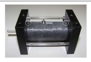
Figure 5-15. Alignment Marks on Pump Cylinder and End Plates
