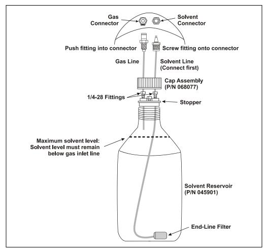
Figure 3-1. Solvent Reservoir Connections
