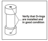
Figure 4-1. Inspecting O-Rings
