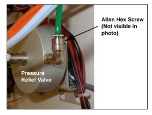
Figure 5-17. Removing the Allen Hex Screw
