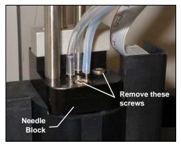
Figure 5-23. Removing the Needle Block Screws
