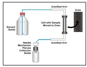
Figure 2-11. Extraction Process: Loading
