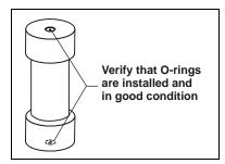
Figure B-10. Inspecting Cell O-Rings
