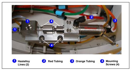
Figure 5-21. Removing the Static Valve
