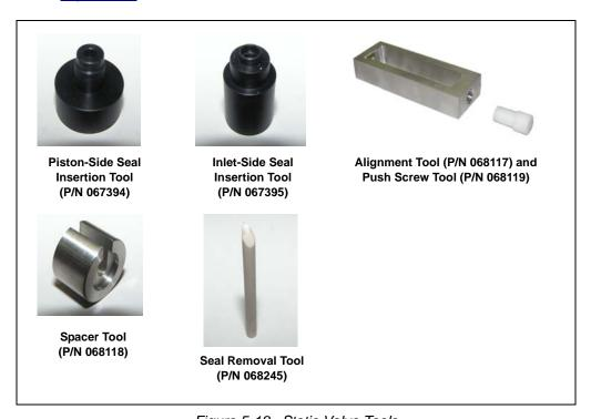
Figure 5-18. Static Valve Tools
