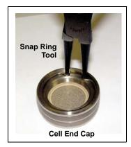
Figure 5-1. Removing the Snap Ring
