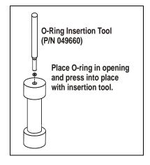
Figure B-11. Installing a Cell End Cap O-Ring
