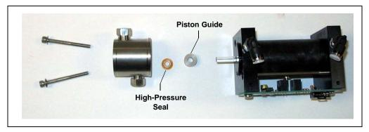
Figure 5-10. Replacing the Dionex ASE 350 Piston High-Pressure Seal
