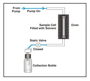
Figure 2-13. Extraction Process: Filling
