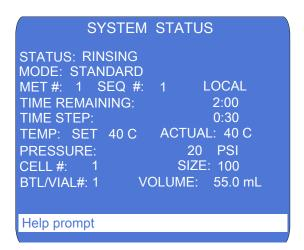
Figure 2-18. System Status Screen: Rinsing
