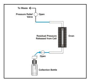
Figure 2-21. Extraction Process: Relief
