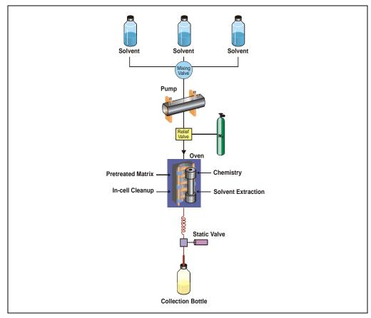
Figure E-1. Schematic of the ASE Process
