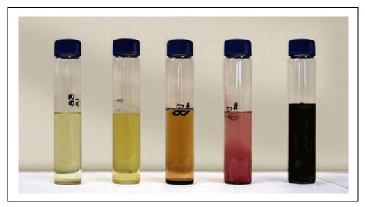
Figure E-3. Selectivity in ASE. The same sample of blueberries was extracted with (from left to right) hexane, DCM, ethyl acetate, acetonitrile, and ethanol
