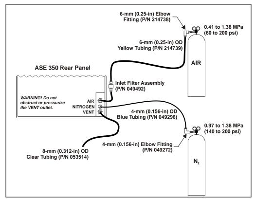
Figure B-1. Dionex ASE 350 Rear Panel Connections
