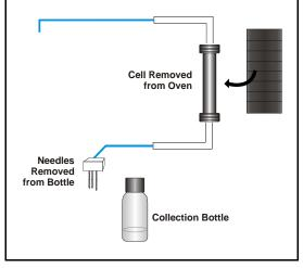
Figure 2-23. Extraction Process: Unloading the Cell
