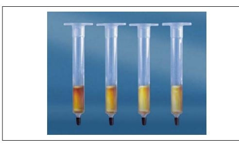
Figure E-4. Residual co-extractives after the ASE extraction of a coffee sample trapped on an SPE cartridge, the ASE cells containing varying from 0 to 6 g Florisil. From left to right: 1) No Florisil in the ASE cell, 2) 2 g Florisil in the ASE cell, 3) 4 g Florisil in the ASE cell, and 4) 6 g Florisil in the ASE cell
