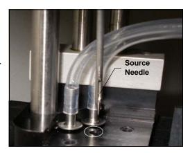
Figure 5-28. Installing the New Source Needle
