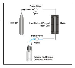
Figure 2-19. Extraction Process: Purging
