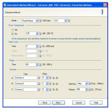
Figure 3-26. Example Method 6: Fixed Volume Mode
