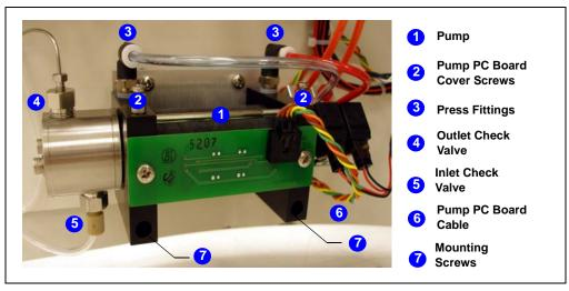
Figure 5-5. Dionex ASE 350 Pump (Shown with PC Board Cover Removed)
