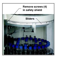
Figure 5-19. Removing the Safety Shield
