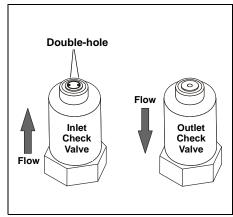
Figure 5-8. Check Valve Assemblies
