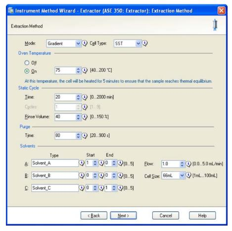
Figure 3-27. Example Method 7: Gradient Mode
