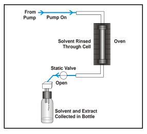
Figure 2-17. Extraction Process: Rinsing
