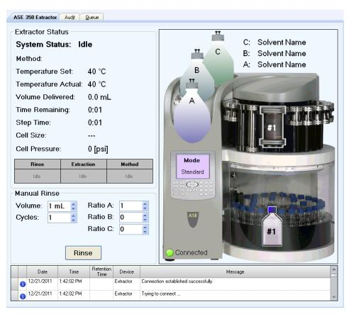
Figure 3-18. Chromeleon Software: Example Dionex ASE 350 ePanel
