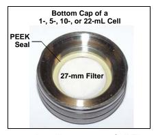
Figure 3-4. Installing a 27-mm Cell Filter
