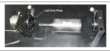
Figure 5-13. Removing the Pump Left End Plate
