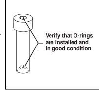
Figure 3-10. Inspecting Rinse Tube O-Rings
