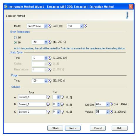
Figure 2-26. Chromeleon Software: Example Extraction Method Page
