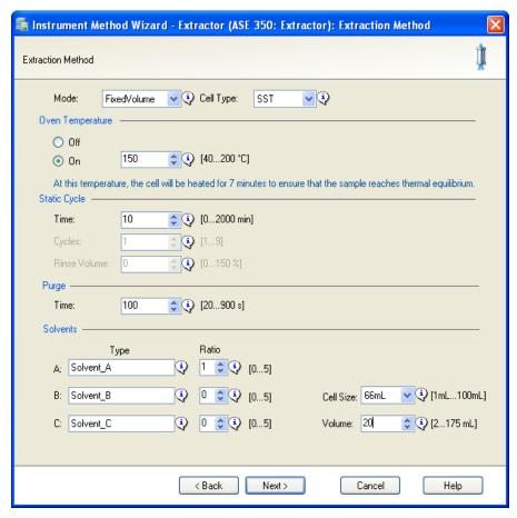
Figure 3-25. Example Method 5: Fixed Volume Mode
