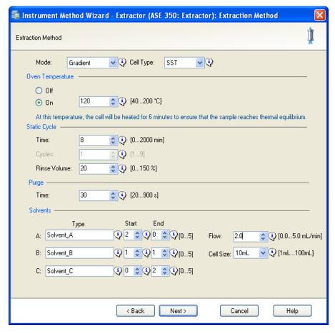
Figure 3-28. Example Method 8: Gradient Mode
