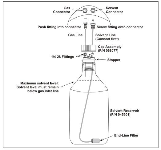
Figure B-7. Solvent Reservoir Connections
