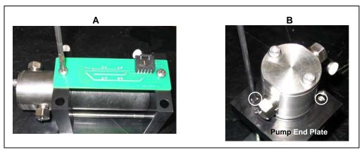
Figure 5-11. Removing the Pump PC Board and End Plate Bolts
