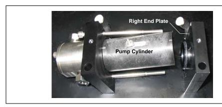
Figure 5-12. Removing the Pump Right End Plate
