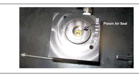
Figure 5-14. Removing the Piston Air Seal
