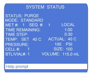
Figure 2-20. System Status Screen: Purging
