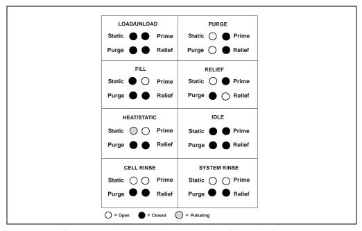
Figure 2-25. Valve Positions During the Extraction Process
