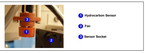
Figure 5-29. Hydrocarbon Sensor
