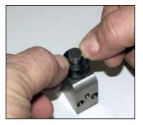
flat in the valve body, with no visible edges. If the seal is damaged, remove it from the valve body and order a replacement seal.
