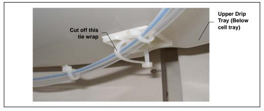
Figure 5-20. Tie Wrap Removal
