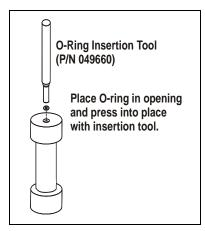
Figure 4-2. Installing a Cell End Cap O-Ring
