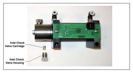
Figure 5-6. Disassembled Dionex ASE 350 Inlet Check Valve
