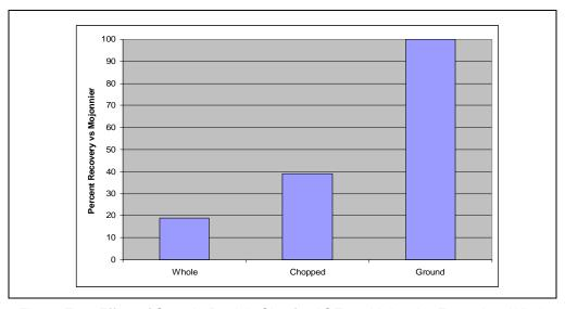
Figure E-2. Effect of Sample Particle Size for ASE vs. Mojonnier Extraction. Whole cheese (0.5 to 1.5 cm size); chopped (2 to 5 mm); ground (mixed thoroughly with diatomaceous earth)
