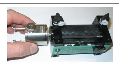
Figure 5-9. Removing the Pump Head
