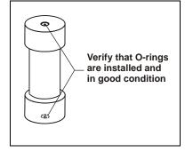
Figure 3-8. Inspecting Cell O-Rings
