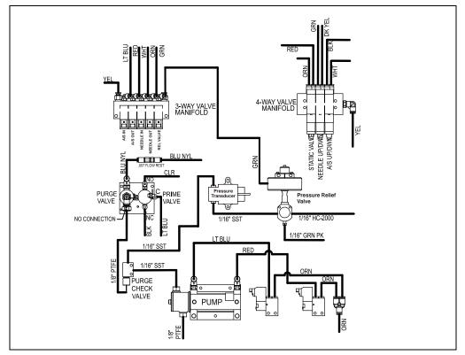
Figure 4-3. Dionex ASE 350 Solvent and Gas Flow Schematic
