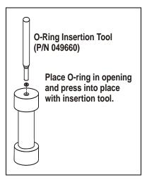
Figure 5-4. Installing a Cell End Cap O-Ring
