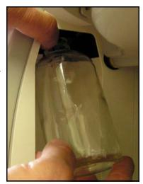
Figure B-9. Installing the Waste Bottle
