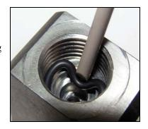
8. Using a cotton-tipped swab (or other tool with a soft tip), thoroughly clean the inside of the valve body. If necessary, moisten the area with IPA (isopropyl alcohol) or acetone to remove all debris, sediment, and precipitates.
