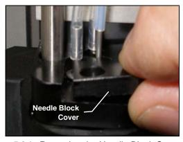
Figure 5-24. Removing the Needle Block Cover
