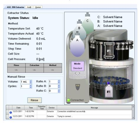
Figure 2-8. Chromeleon Software: Example Dionex ASE 350 ePanel
