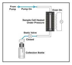
Figure 2-15. Extraction Process: Heating and Static
