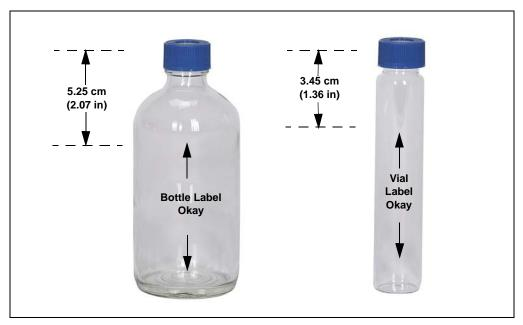
Figure 3-11. Placement of Collection Vessel Labels
