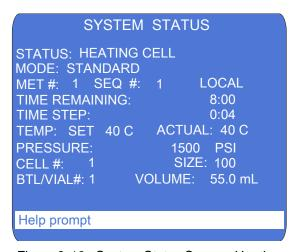
Figure 2-16. System Status Screen: Heating
