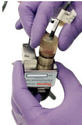
Figure 100. Installation of the pH-Ag/AgCl reference electrode in the reference electrode well
