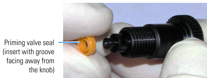
Figure 88. Priming valve and seal
