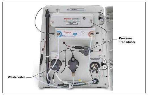
Figure 5-1. Dionex Easion Interior Components
