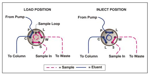
Figure 2-6 shows flow schematics for the valve.
