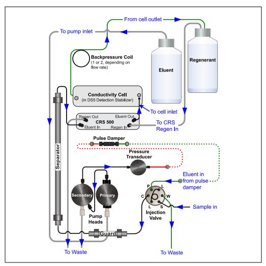
Figure 5-2. Dionex Easion Flow Schematic
