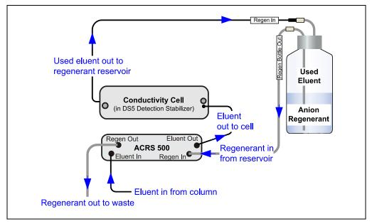
Figure 2-7. Anion Displacement Chemical Regeneration (DCR)
