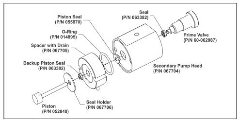
Figure 5-7. Secondary Pump Head
