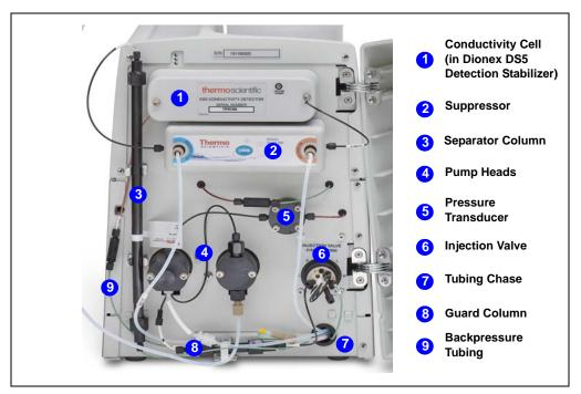
Figure 2-2. Dionex Easion Component Mounting Panel
