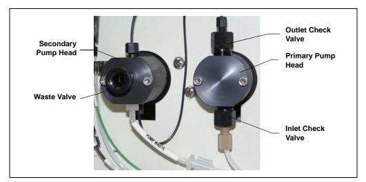
Figure 2-5. Dionex Easion Pump Components
