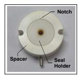
3. Insert a thin object (for example, the straightened end of a paper clip) into the spacer and carefully pry the backup piston seal out of the spacer. **Be careful not to scratch the spacer**.
