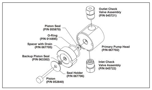
Figure 5-6. Primary Pump Head
