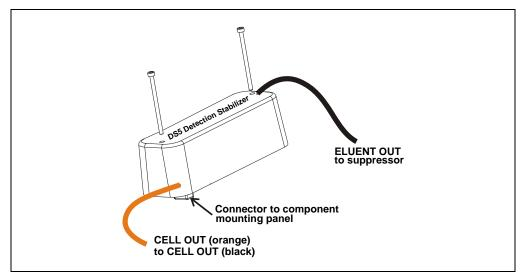
Figure 5-10. Conductivity Cell Assembly
