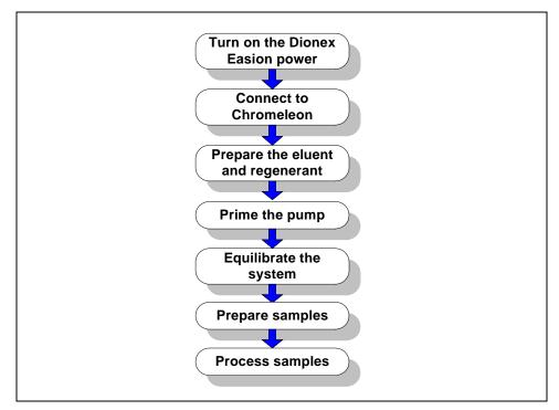
Figure 3-1. Dionex Easion Operation Flow Chart
