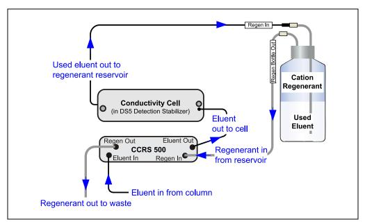
Figure 2-8. Cation Displacement Chemical Regeneration (DCR)
