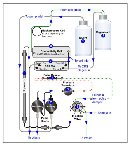
Figure 2-4. Dionex Easion Flow Schematic
