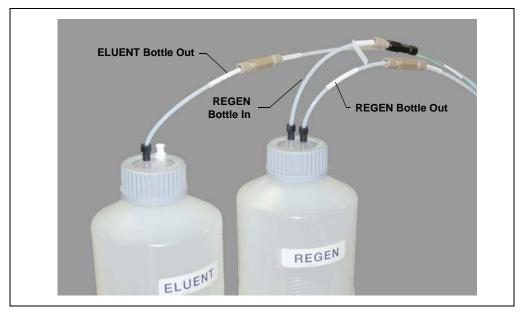
Figure 3-2. Eluent and Regenerant Bottle Liquid Line Connections
