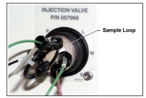
Figure 5-3. Dionex Easion Injection Valve
