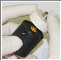
5. To seat the seal, push down on the spacer until it is flush with the pump head. A clicking sound indicates that the seal is correctly seated.
