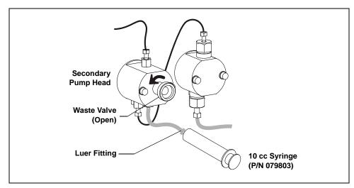
3. Connect a 10 cc syringe (P/N 079803) to the luer fitting (see Figure 3-4).
