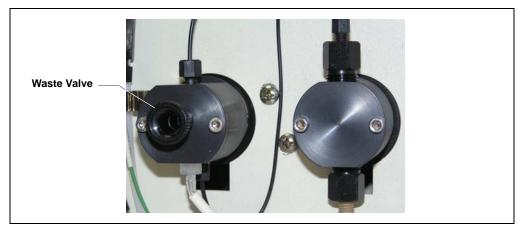
Figure 5-8. Waste and Priming Valves
