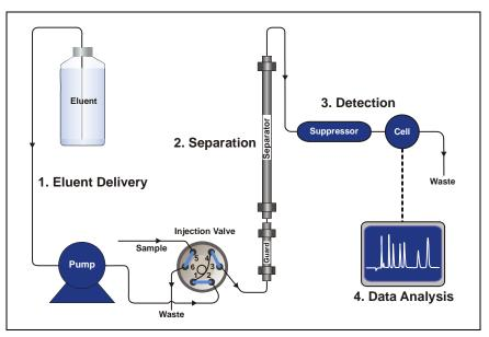
The IC analysis consists of four stages (see Figure E-1).
