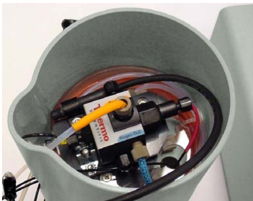
Figure 88. CR-TC Installed in Holder
