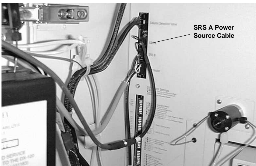
Figure 104. The DX-120 SRS A Power Source Cable
