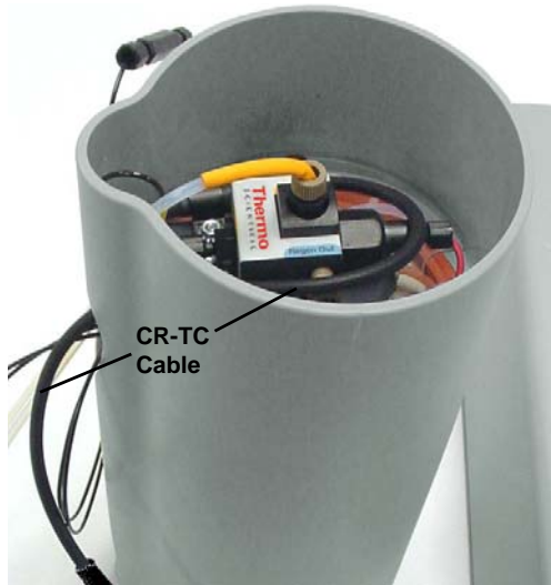
Figure 89. Installing the CR-TC
