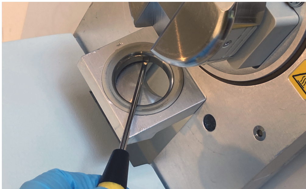
Figure 102. Using a small flathead screwdriver to loosen the drain ring
