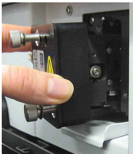
Fig. 17: Inserting the flow cell
