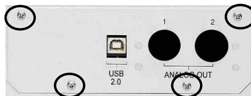
Fig. 9: Screws on the access panel
