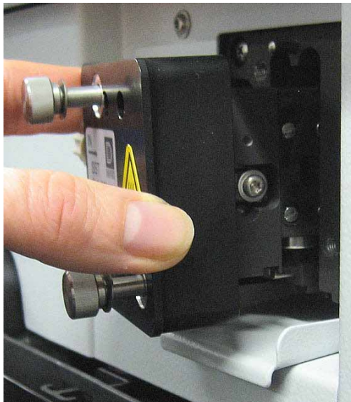
Fig. 39: Inserting the flow cell
