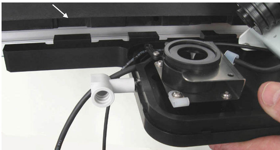
Fig. 8: Installing the flow cell carrier
