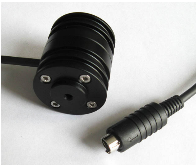
Fig. 3: Conductivity flow cell with connection cable
