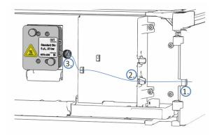
Figure 23: Connecting the inlet capillary from the column compartment (example)
