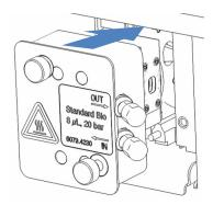
Figure 37: Inserting the flow cell
