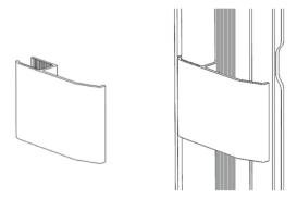
Figure 17: Tubing bracket (left), tubing bracket installed (right)
