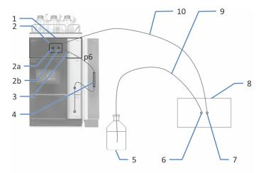
Figure 31: Calculating the pressure at the inlet port of the flow cell in your used system configuration (here with second detector)
