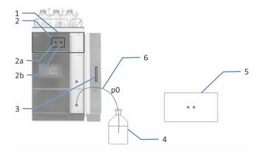
Figure 27: Measuring the backpressure of the waste line
