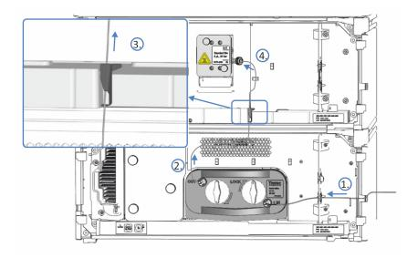
Figure 24: Connecting the inlet capillary from the diode array detector (example)
