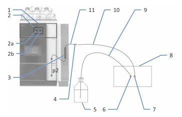
Figure 29: Determining the backpressure of a second detector (example)
