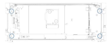
Figure 40: Captive screws on the slide-in module
