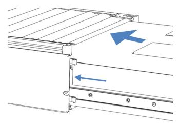
Figure 42: Inserting the slide-in module
