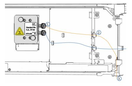
Figure 26: Connecting the detector waste line
