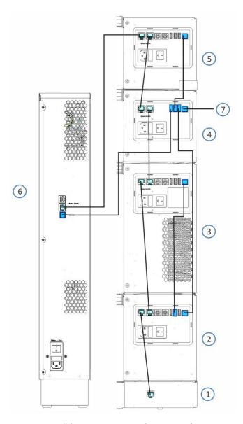
Figure 13: Cable connections in the Vanquish system with fluorescence detector and diode array detector (example)
