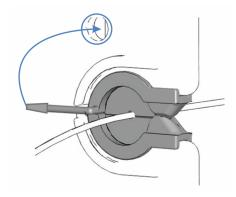
Figure 19: Securing the partition panel plug with slit
