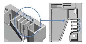
Figure 16: Tubing chase with tubing guides (left: view from inside, right: view from top)
