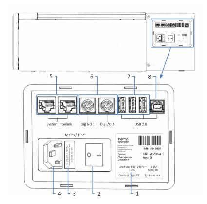
Figure 12: Electrical connectors on the right side of the detector
