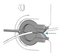
Figure 20: Capillary installed in the plug with slit
