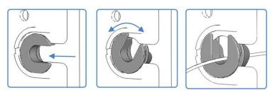
Figure 21: Using the rotating plug
