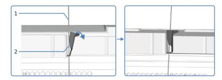
Figure 25: Securing the capillary behind the capillary clip on the leak tray
