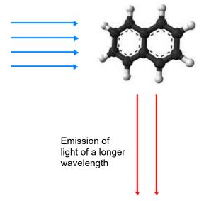
Figure 2: Simplified presentation of a molecule emitting light (fluorescence)
