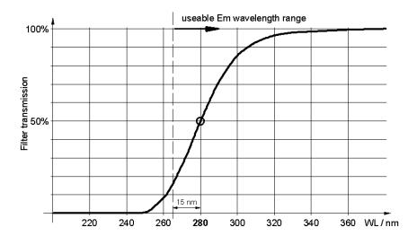
Figure 35: Transmission behavior of the 280 nm filter
