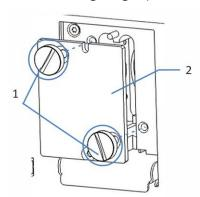
Figure 36: Installing the flow cell cover
