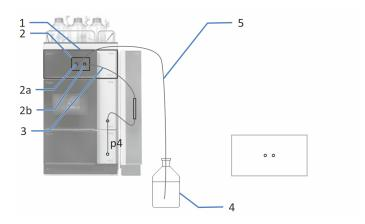
Figure 30: Measuring the backpressure of the flow cell including column, detector inlet capillary and waste line
