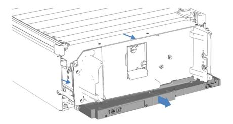
Figure 41: Pulling out the slide-in module
