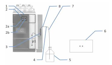
Figure 28: Measuring the Vanquish system backpressure (without flow cell)
