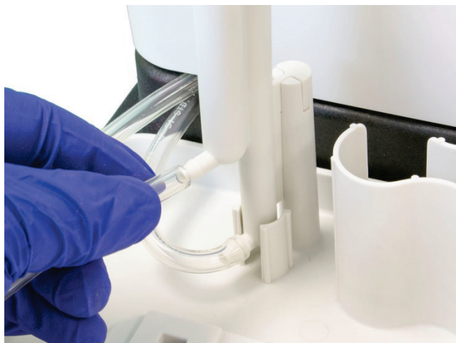
Figure 17 Connecting the Rinse Station Drain
