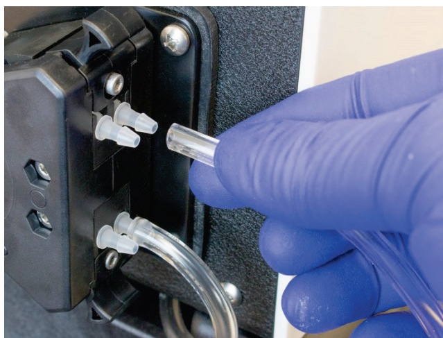
Figure 16 Connecting the Rinse Solution Source to the Pump
