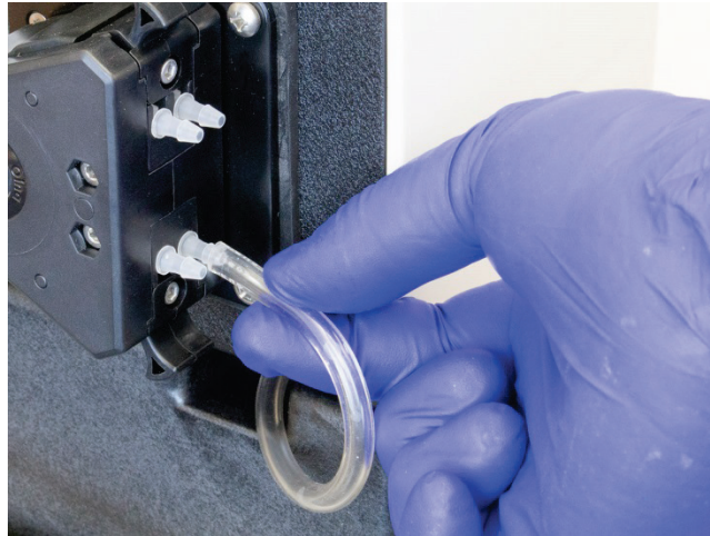
Figure 14 Connecting the Pump Output
