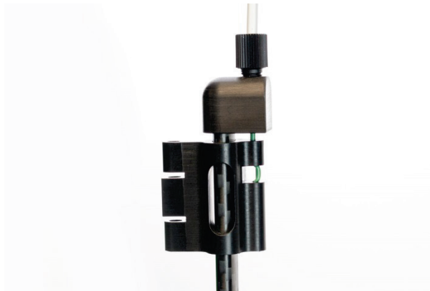
Figure 9 Z-Drive at Top Position With Gap
