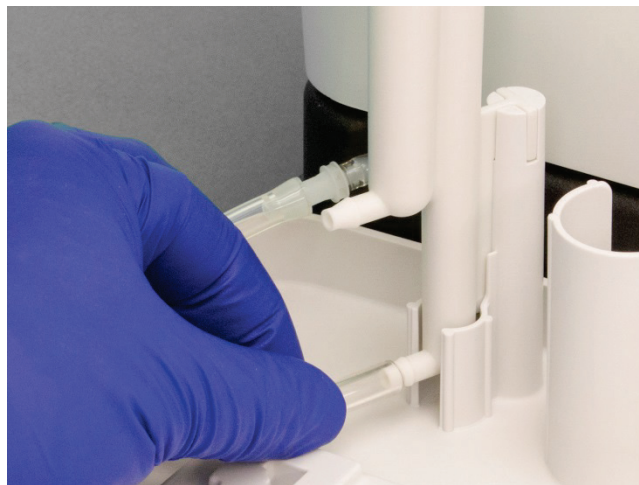
Figure 15 Connecting the Rinse Station Input
