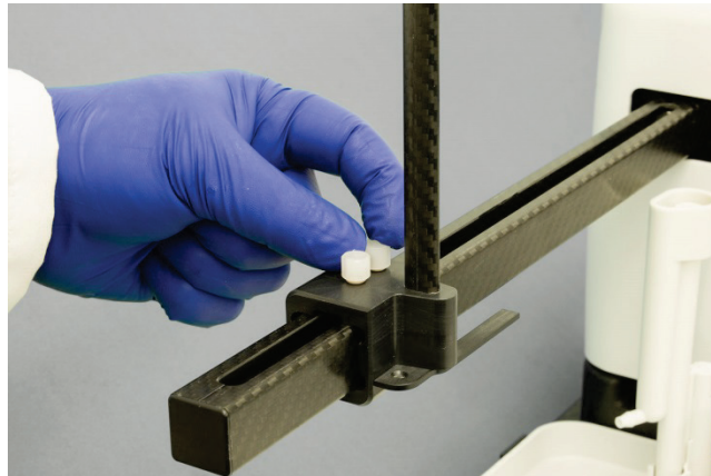
Figure 6 Securing the Z-Drive
