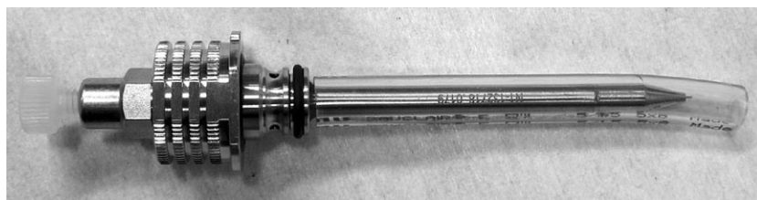
Figure 29: Nebulizer with protective tubing and inlet plug
