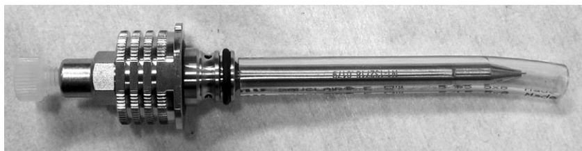
Figure 12: Nebulizer with protective tubing and plug on the flow inlet
