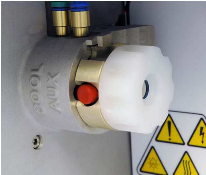
Figure 2-6. Insertion of the torch assembly into the box
