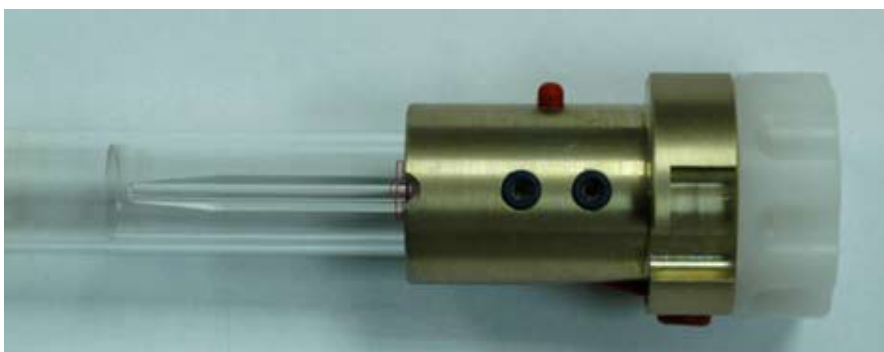
Figure 2–5. Insertion of centre tube into torch assembly
