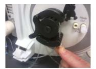
4. Screw the green valve fitting into port 5 on the valve head.
