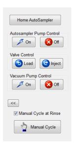
Figure A-14. Manual control features in external Sprint Valve Configurator
