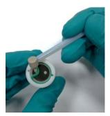
**Figure 8-4.** Removing green O-ring
