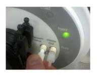
7. Attach the vacuum pump waste tubing to the waste out connector of the iCAP 7000 Plus Series ICP-OES.
