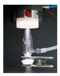
**Figure 3-9.** Sheath gas introduced between spray chamber and torch
