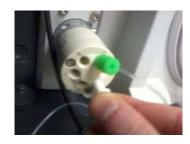
6. Screw the other end of the fitting tube into the vacuum valve connector of the iCAP 7000 Plus Series ICP-OES.
