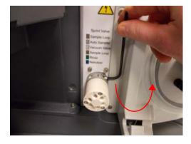
Figure A-24. Tightening the locking collar
