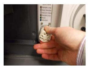
Figure A-23. Checking the valve seat
