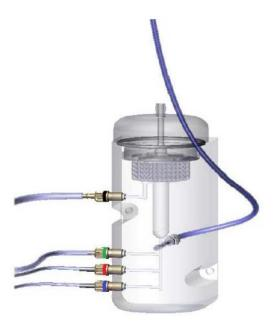
Figure B-4. Integrated hydride generation kit
