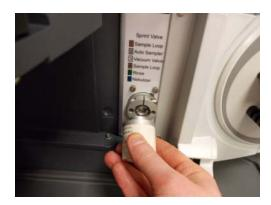
Figure A-22. Inserting the valve
