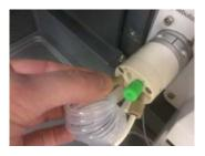
10. Screw the fitted nebulizer tube into port 6.
