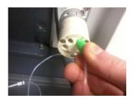
5. Take the white valve fitting tube and attach one end to port 3 on the valve head.
