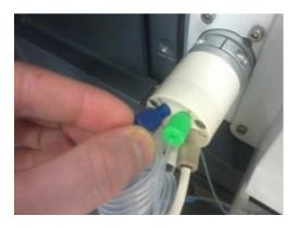
Figure A-26. Reconnecting the tubing
