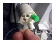
9. Attach the sample loop into ports 1 and 4 of the valve head (this is the same as the loop provided in the Field Service Test Kit).
