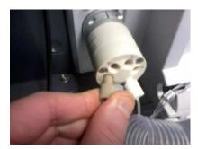
**Figure A-20.** Removing the tube connectors
