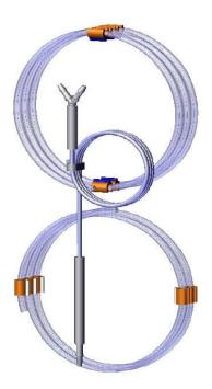
Figure 3-4. Internal Standards mixing kit
