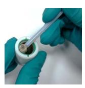
**Figure 8-5.** Inserting green O-ring
