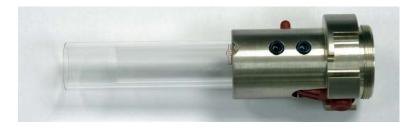
Figure 6-14. Radial torch assembly
