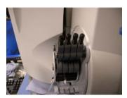
**Figure 7-2.** Peristaltic sample pump
