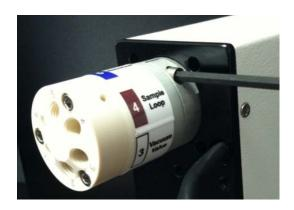
Figure A-17. Loosening metal collar on Sprint Valve
