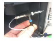
12. In case that a 7-port valve is used, screw the yellow internal standard fitting into port 7 in the center of the Sprint Valve.
