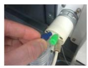
11. Attach the other end on the nebulizer line and the nebulizer gas fitting onto the nebulizer.
