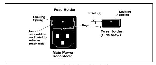
Figure 5-4. Main Power Fuse Holder
