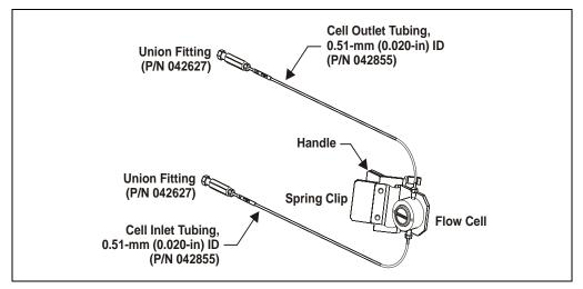
Figure 2-7. Semi-Preparative Flow Cell Assembly
