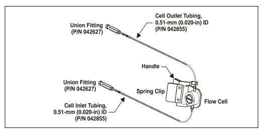
Figure B-2. Semi-Preparative Flow Cell Connections
