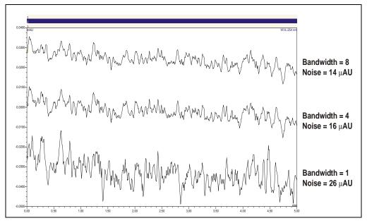
Figure 3-6. Effect of Bandwidth on Baseline Noise
