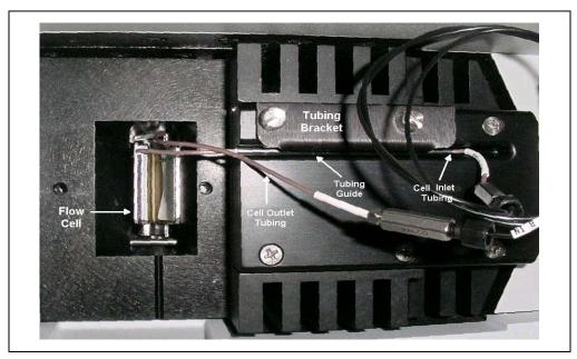
Figure 5-1. Removing the Flow Cell from the Optical Bench (Flow cell cover not shown)
