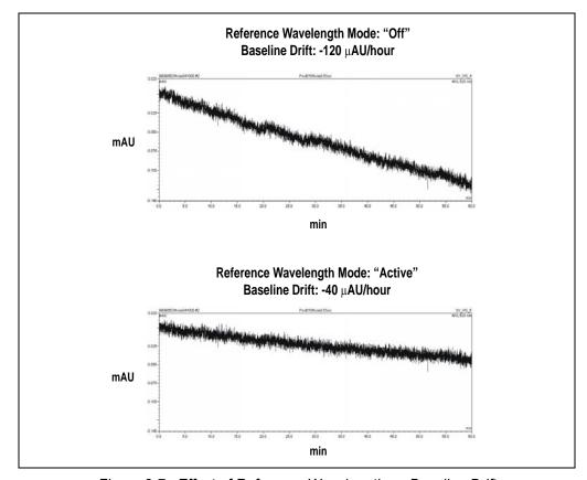
Figure 3-7. Effect of Reference Wavelength on Baseline Drift
