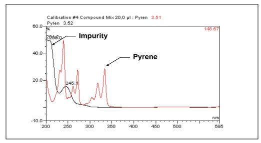
Figure 1-3. Spectra of Pyrene and an Impurity
