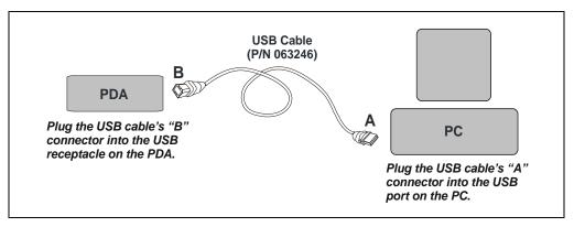
Figure B-5. Dionex PDA Connected Directly to the Chromeleon PC
