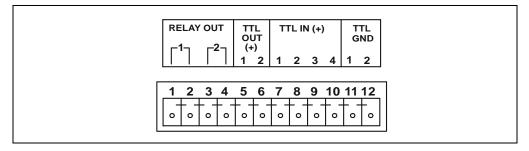
Figure B-4. Relay and TTL Connector
