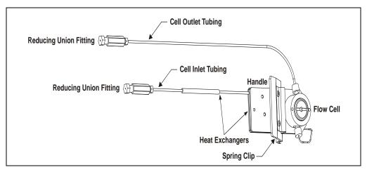
Figure 2-6. Semi-Micro Flow Cell Assembly
