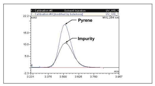
Figure 1-2. Overlay of Pyrene and an Impurity
