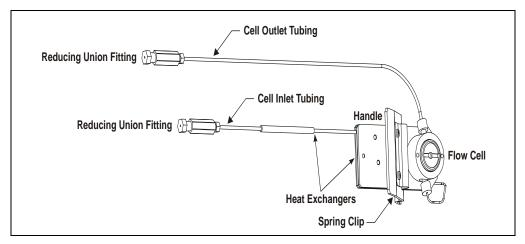
Figure 2-5. Standard Flow Cell Assembly
