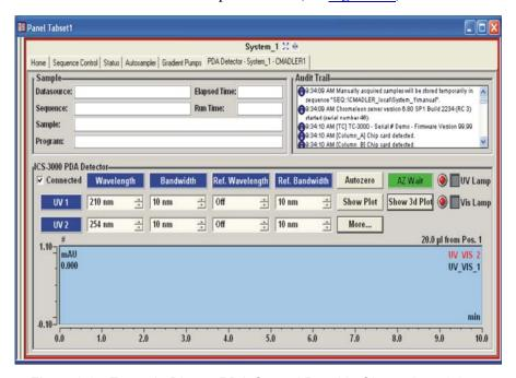
Figure 3-2. Example Dionex PDA Control Panel in Chromeleon 6.8
