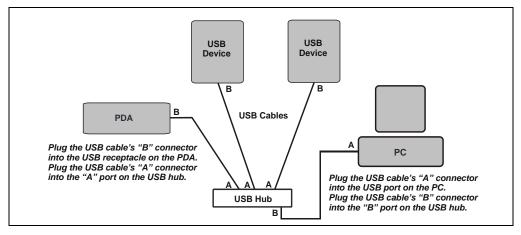
Figure B-7. Example USB Connections: Modules Connected to an External Hub
