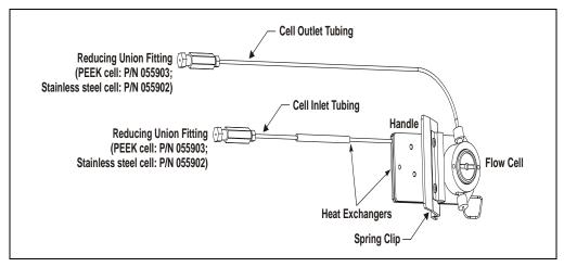
Figure B-1. Standard or Semi-Micro Flow Cell Connections
