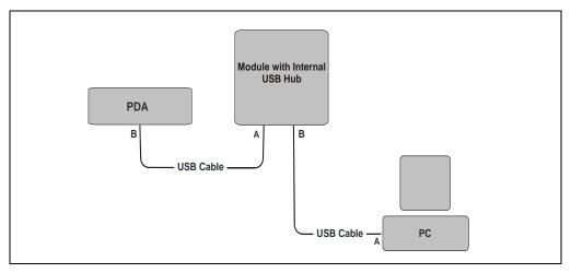
Figure B-6. Example USB Connections:
