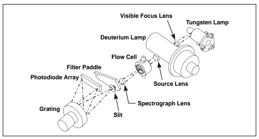
Figure 2-4. Dionex PDA Optical System
