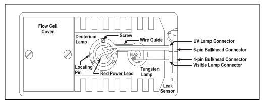
Figure 5-3. Lamp Connections
