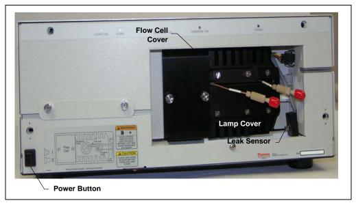
Figure 2-3. Dionex PDA Inside Front Panel
