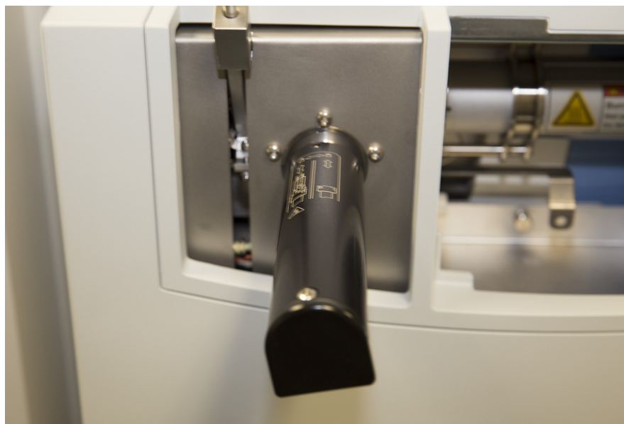
Figure 6-7. Raising the Vacuum Interlock Handle
