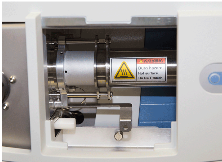
Figure 6-18. Closed MS Transfer Line
