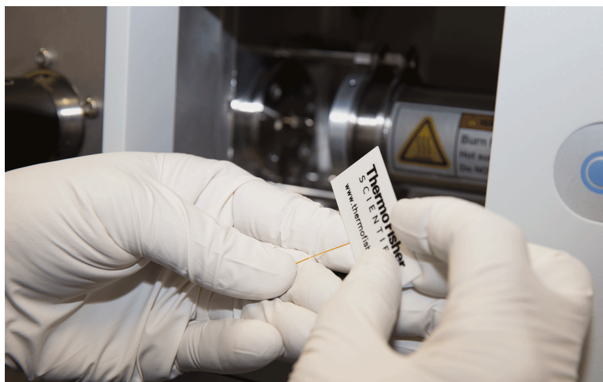
Figure 6-13. Scoring and Cutting the Column
