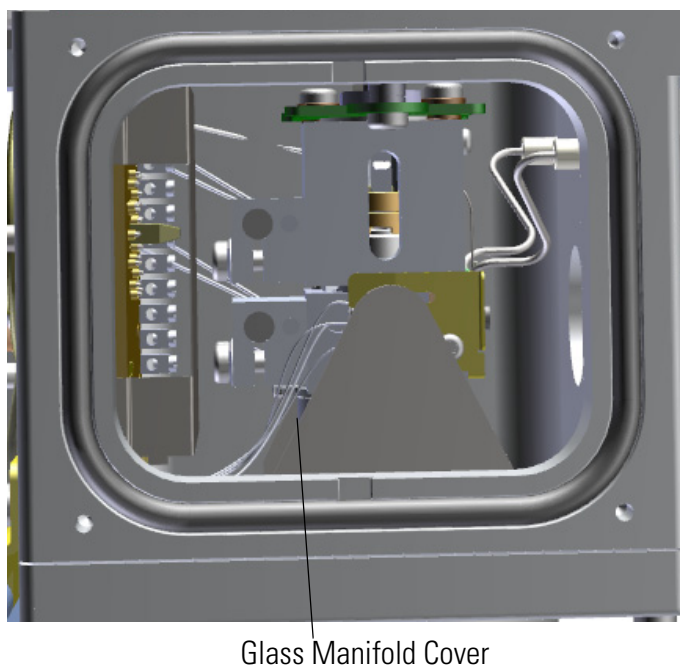
Figure 8-41. Locating the Glass Manifold Cover
