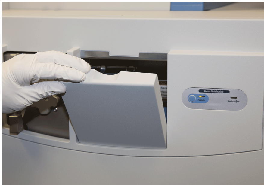
Figure 8-35. Opening the front panel
