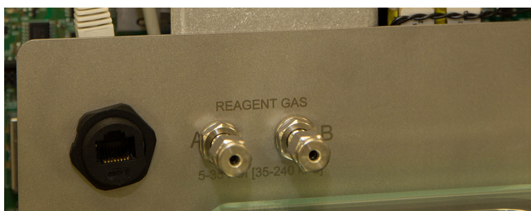
Figure 5-8. Connecting the CI gas supply
