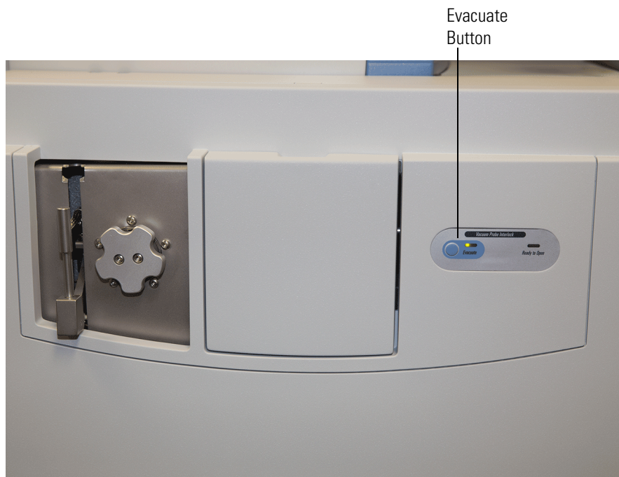
Figure 8-30. Evacuating the Instrument
