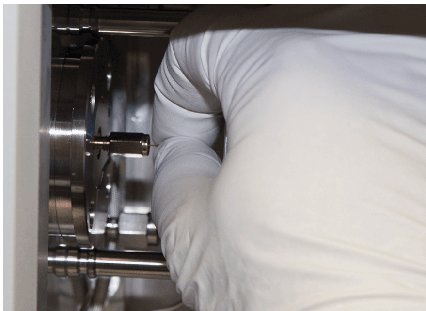
Figure 6-15. Inserting the Column into the MS Transfer Line
