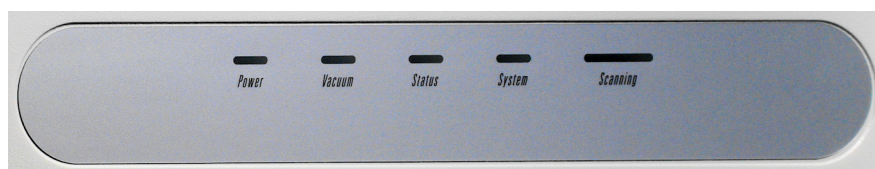
Figure 3-2. System status LEDs
