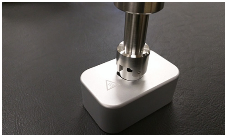
Figure 6-4. Attaching the Source Plug to the Source Exchange Tool
