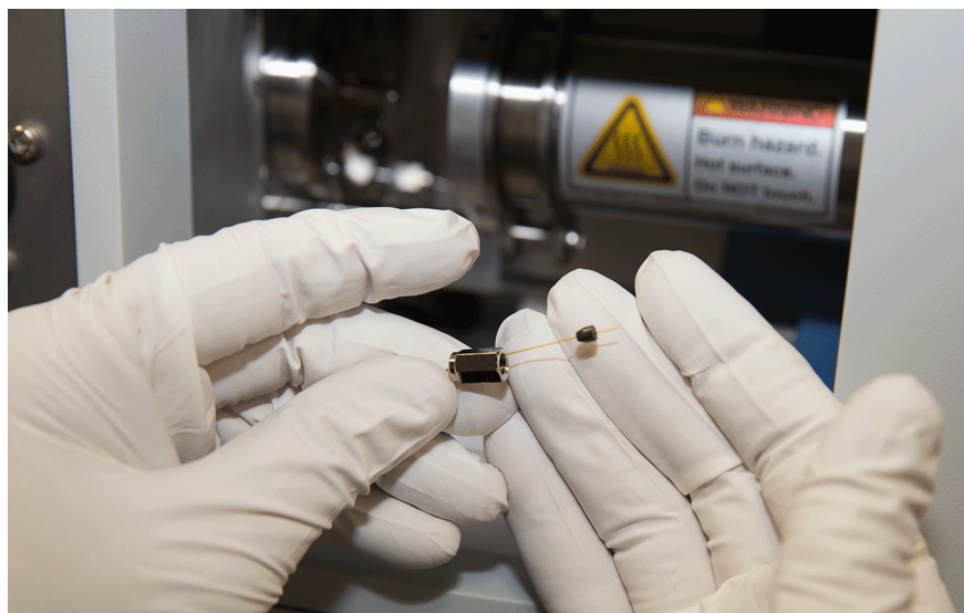
Figure 6-12. Inserting the Column through the Nut and Ferrule
