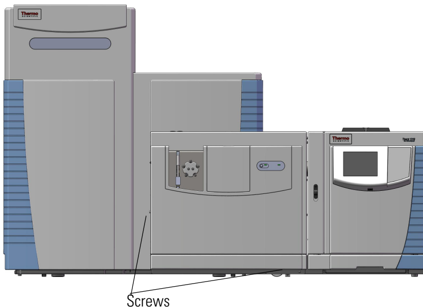
Figure 8-38. Locating the Screws on the Front Panel
