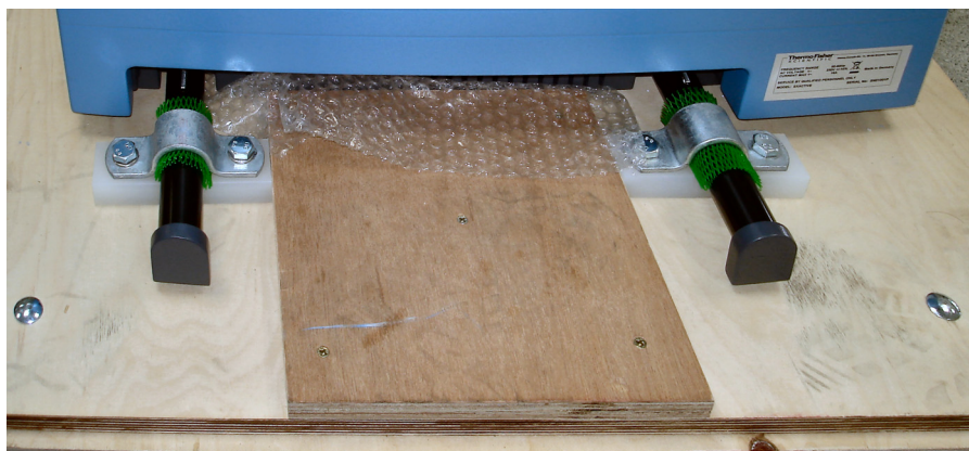
Figure 5-2. Handles, fixed on the transport pallet
