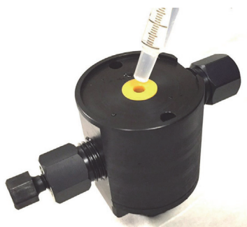
Figure 33. Filling the pump head cavity with deionized water
