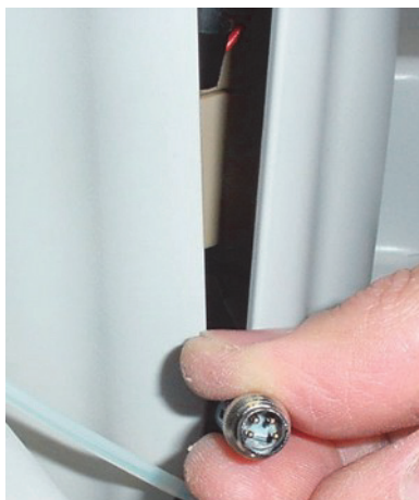
Figure 63. Connecting the Dionex EGC electrical cable
