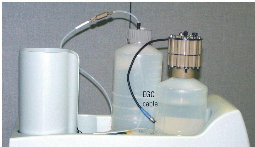
Figure 61. Dionex EGC in the service area
