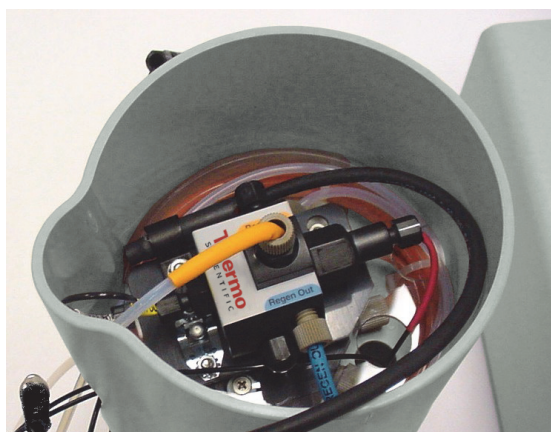
Figure 68. Dionex CR-TC installed in Dionex EGC holder
