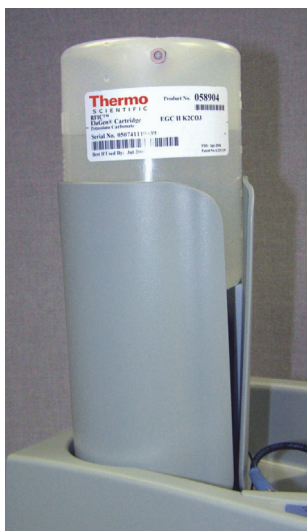
Figure 62. Dionex EGC installed in the holder
