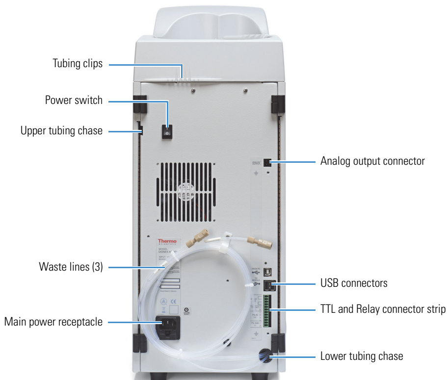
Figure 6. Dionex Aquion RFIC rear panel
