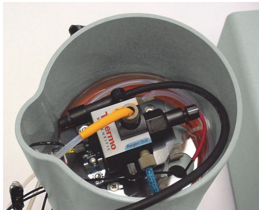
Figure 80. Dionex CR-TC installed in Dionex EGC holder
