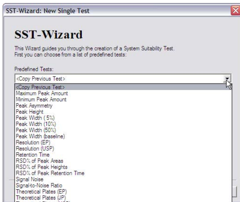
FIGURE 3-16: Start of the wizard for the SST parameters where a predefined test can be selected from the drop-down menu.
