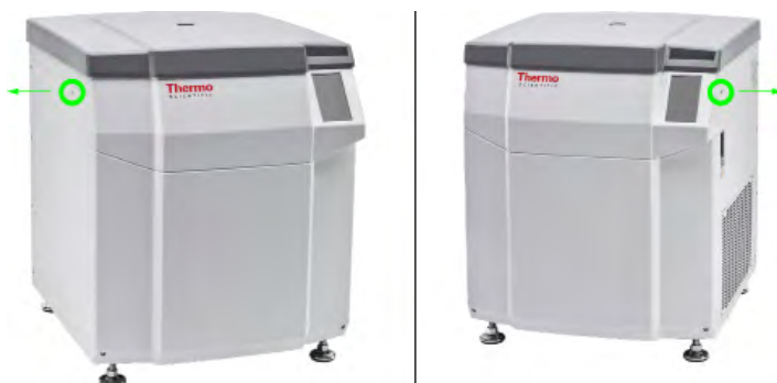
Figure V-2: Position of the mechanical emergency door release
