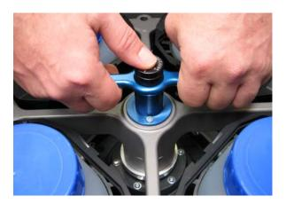
Figure 2. Removing the Rotor
