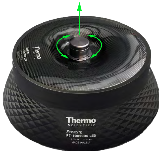
Figure III-11: Remove rotor lid from rotor body
