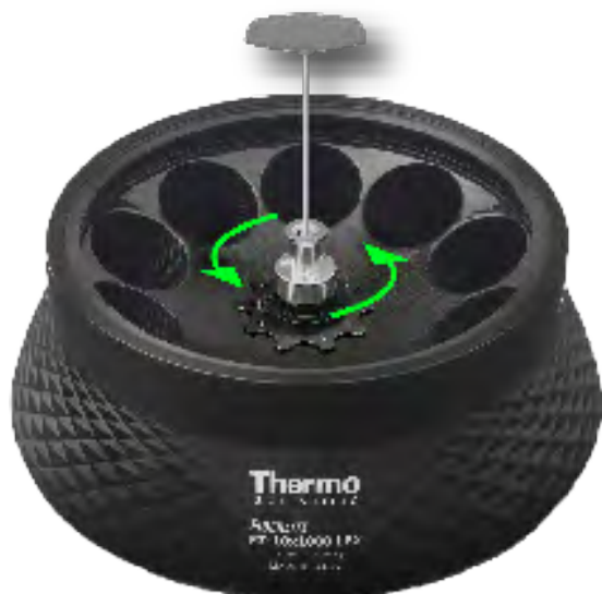
Figure III-12: Disengage the rotor locking screw from drive shaft
