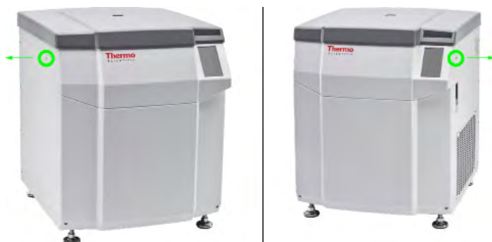
Figure V-2: Position of the mechanical emergency door release
