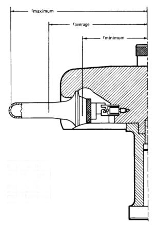
Figure 3-1. AH-629 Rotor Cross Section Showing Radial Distances
