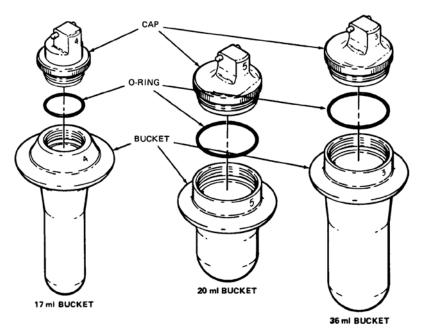
Figure 3-2. Cap and Bucket Assembly
