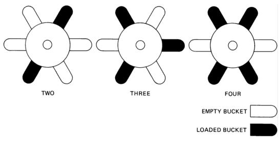
Figure 3-3. Rotor Balancing
