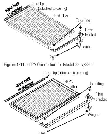
Figure 1-12. HEPA Orientation for Model 3310/3311
