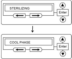
Figure 8-4. Cool Phase in Sterilization Cycle
