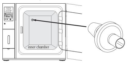
Figure 1-10. Access Port Filter Installation
