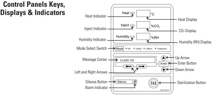
Figure 1-3. Control Panel Components
