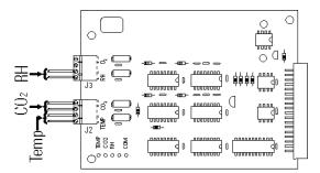
Figure 9-4. Conductors on Analog Output Board
