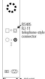
Figure 9-2. RS485 Connector location
