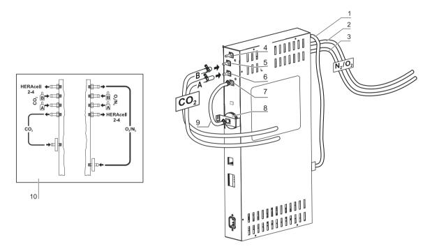
Figure 4-14. Combined CO<sub>2</sub>/O<sub>2</sub>/N<sub>2</sub> Connection with Gas Monitoring System (Optional)
