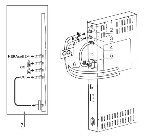
**Figure 4-13.**  $CO_2$  Connection with Gas Monitoring System (Optional) The supplied gas pressure hoses feed the gas from the central gas supply system to the device. Devices with  $CO_2$  connections that are equipped with the optional gas monitoring system are connected according to the connection diagram (7/Figure 4-13).
