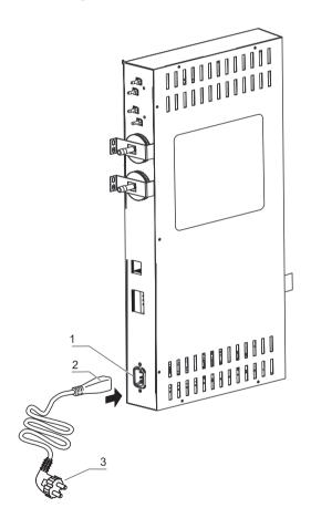
Figure 4-15. Power Supply Connection
