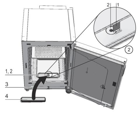
4. Insert the pre-filter (4/Figure 4-2) into the water reservoir cover panel.
