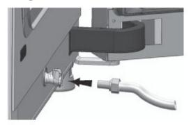
Figure 3-15. Fill and Drain Valve Incubator
