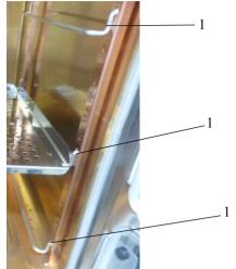
Insert the shelf supports (1) in the lower, center and upper **rectangular** holes of the support rails. In the upper and center position place the perforated shelves with the unseparated guiding rails.
