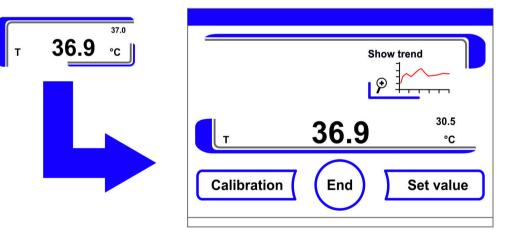
Figure 6-7. Temperature Display Field and Temperature Selection Menu
