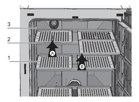
Figure 4-10. Installation of Split Inserts
