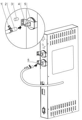
Figure 4-11. Installing Gas Pressure Hoses
