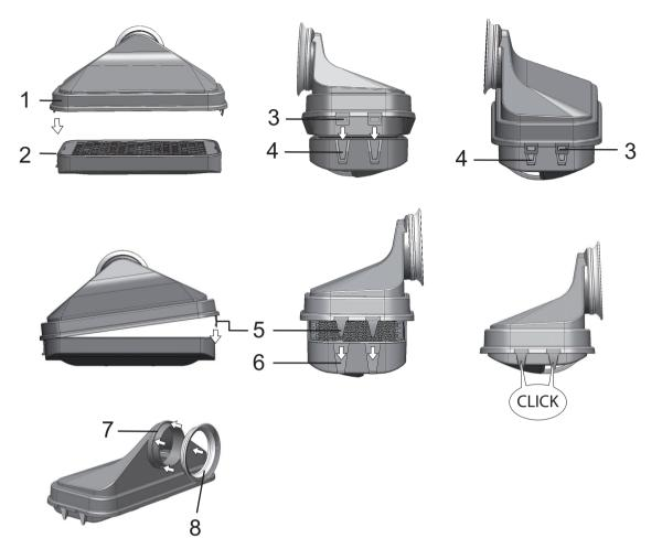
Figure 9-7. Installing the HEPA-Filter
