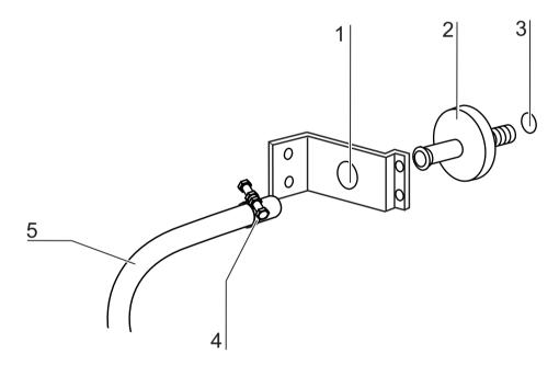
Figure 9-8. Gas Inlet Filter Installation
