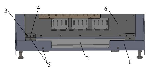
Figure 2-10. Fixing device on support stand with counter weight
