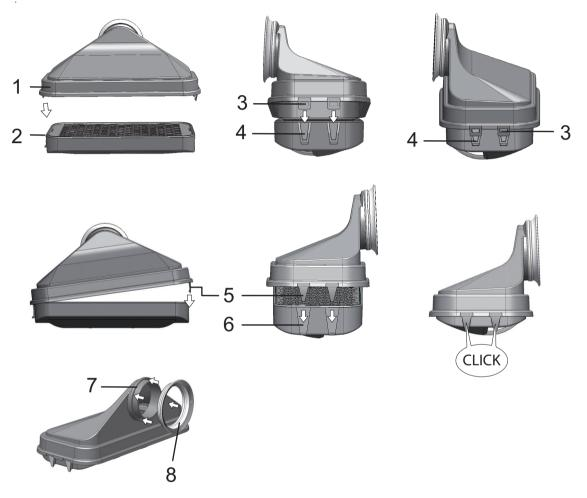
Figure 3-4. HEPA-Filter and Airbox
