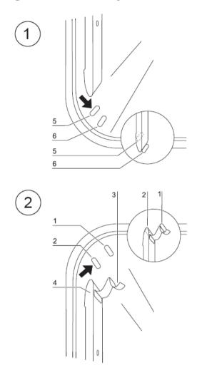
Figure 4-8. Support Rail Installation/Removal
