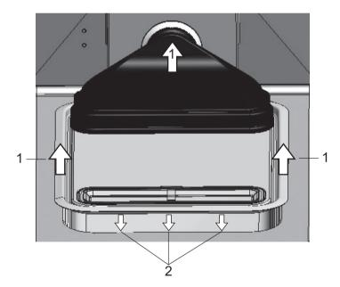
Figure 4-7. Installing the Airbox
