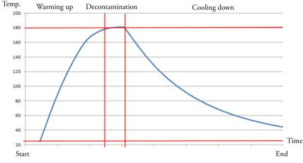
Figure 8-4. Decontamination Routine Phases
