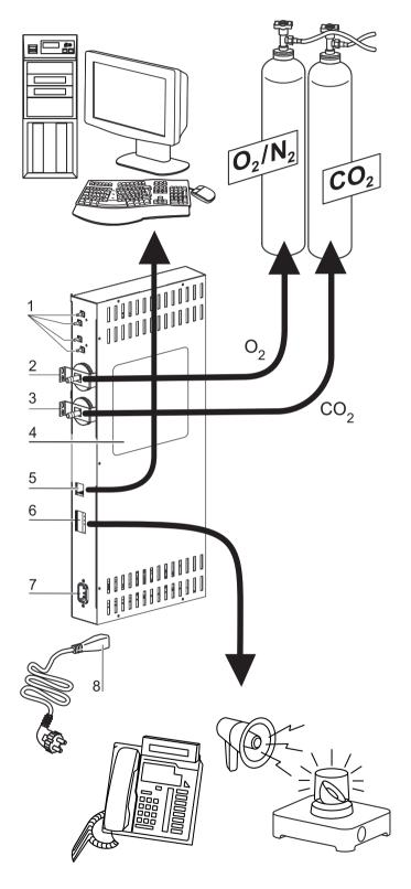
Figure 3-9. Interfaces (Right Side of Control Box)
