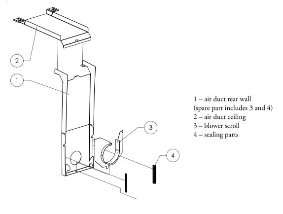
Figure 4-4 shows lists the parts that make up the air duct assembly installed in the inner chamber.
