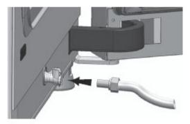
Figure 5-2. Fill and Drain Valve Incubator
