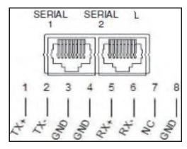
Figure 11. Controller serial ports and RS-485 4wire pin diagram
