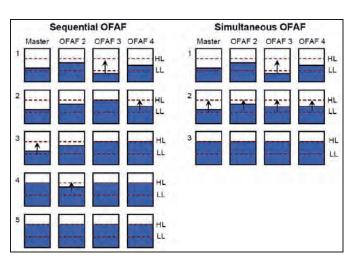
Figure 13. Diagram showing difference between Sequential and Simultaneous OFAF
