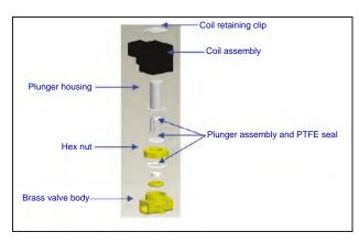
**Note:** If the brass valve body requires replacing, the freezer plumbing will need to be disassembled and the entire valve replaced (PN 14224611S). It is typically easier to start disassembling the plumbing assembly beginning at the fill tee for fill valve replacement or the gas bypass muffler for gas bypass valve replacement.
