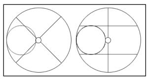
Figure 1. Top-view of HE Freezer showing offset neck and P and R turn-trays
