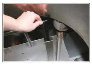
Level dip stick inserted to measure the physical liquid nitrogen level
