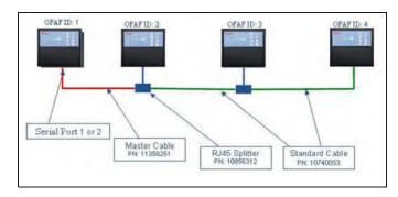
Figure 14. Diagram showing a typical OFAF network setup
