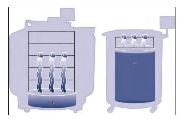
Figure 2. Illustration showing LN<sub>2</sub> as the refrigerant. Left: LN<sub>2</sub> below the storage space naturally boils off and cools the freezer. Right: LN<sub>2</sub> resides in the freezer storage space.
