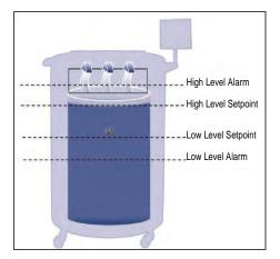
Figure 4. Example of automatic level control parameters
