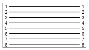
Figure 16. Standard reverse RJ-45 network cable configuration. Numbering as viewed from side of the connector opposite latch.
