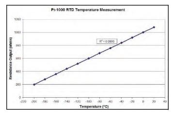
Figure 5. Platinum's linear relationship between temperature and resistance
