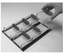
2. Pour enough compatible running buffer into the unit to fill the chamber and completely cover and submerge the gel. Correct buffer level is clearly marked on the units side wall as "FILL LINE". See Recommended Running Conditions for approximate buffer volumes needed for your unit. Too little buffer may cause the gel(s) to dry out during the run, while excess buffer may decrease DNA mobility and cause band distortion.
