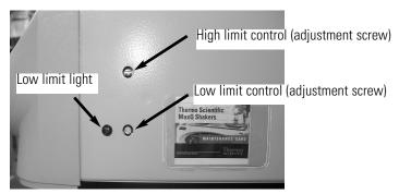
**Figure 5-3.** Control Limit Locations (Refrigerated Unit Shown)
