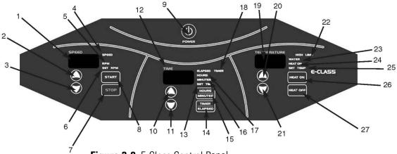
Figure 3-2. E-Class Control Panel
