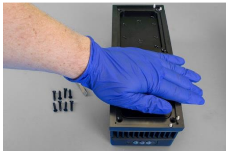
Fig. 18: Pressing the new bezel into place
