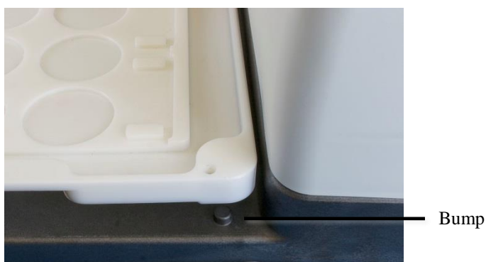
Fig. 34: Installing the spill tray
