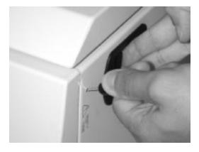
While pressing up with your finger, to press down with the unlocking tool, pull the lid lever toward you: the lid opens upwards.
