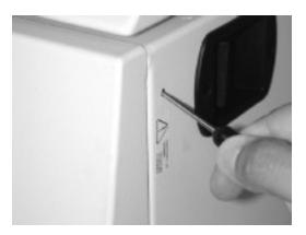
Insert the unlocking tool horizontally into the hole on the right hand side of the instrument.
